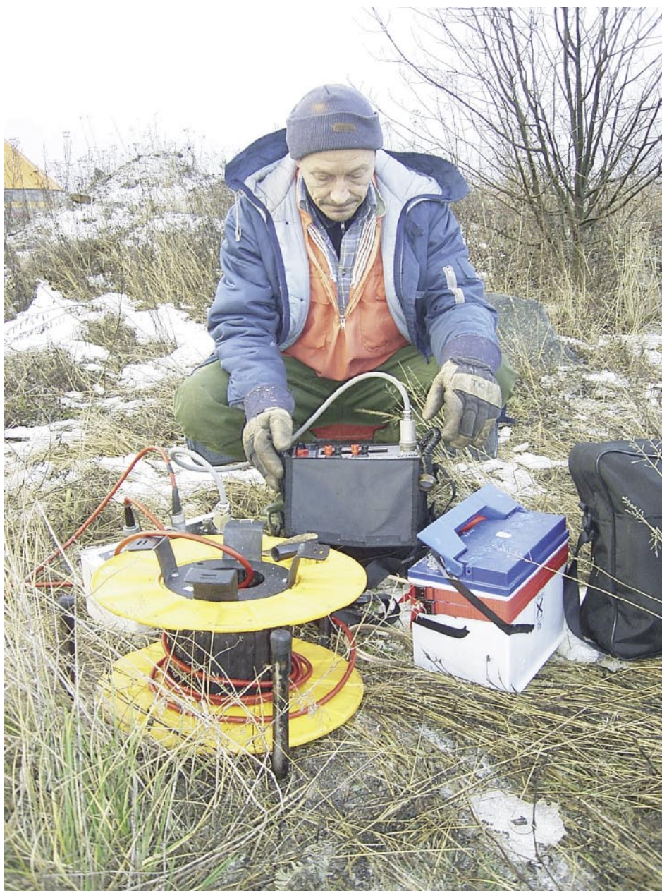
Figure 3-1. Measurements of the resistivity with the Lund Imaging System (ABEM AB).
