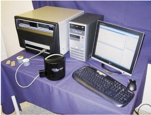
Figure 3-1. Hot disk Thermal Constants Analyser.
