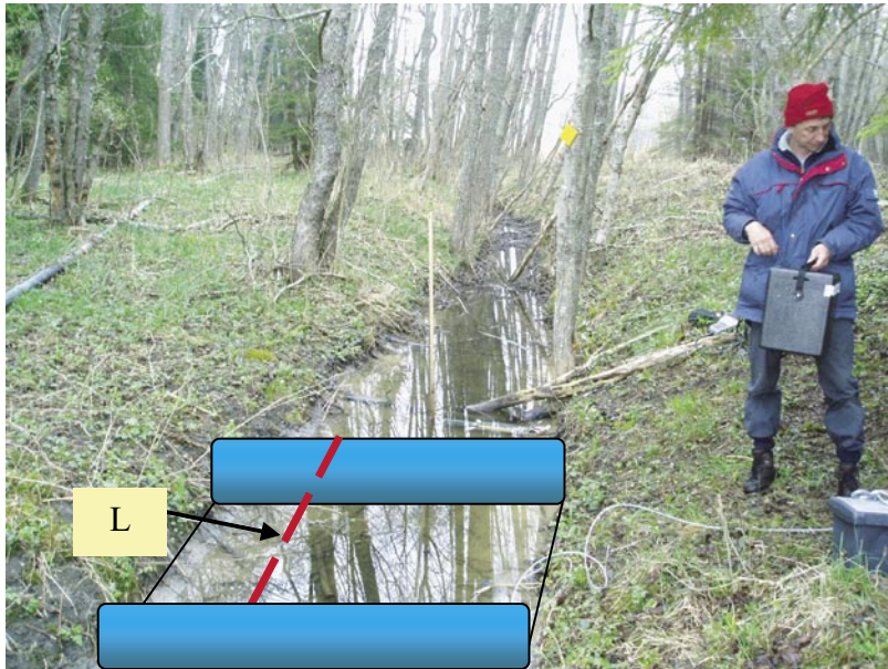
Figure 3-1. Schematic illustration of the float method used for the manual discharge measurements (PFM000073 South of Bredviken) /From Nilsson et al. 2003/.
