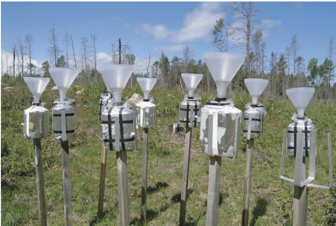
Figure 3-1. The ten samplers are placed within an area of 3x3 m in an open and undisturbed environment (PFM002564).
