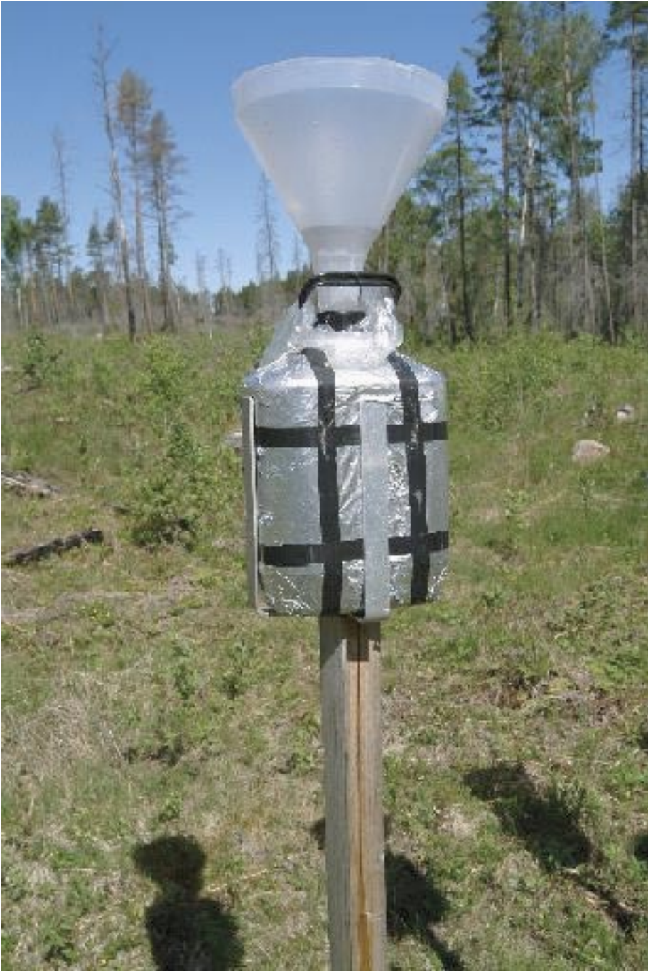
Figure 3-2. Precipitation sampler used in summer time.
