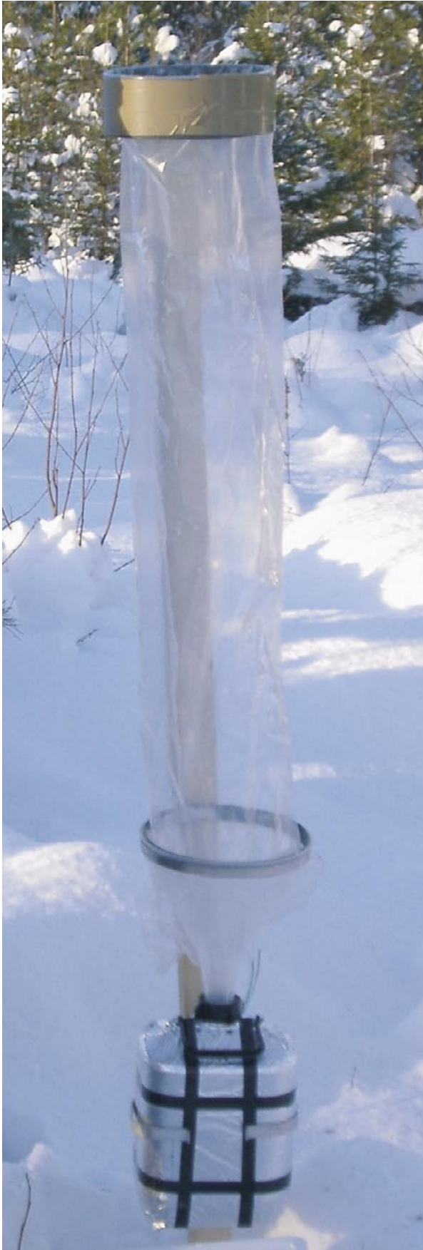
Figure 3-3. Precipitation sampler used in winter time.
