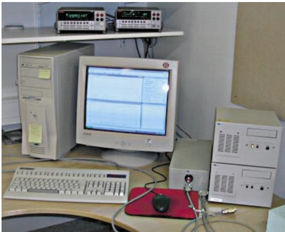
Figure 3-1. TPS-apparatus with source meter, multi-meter, bridge, and computer.
