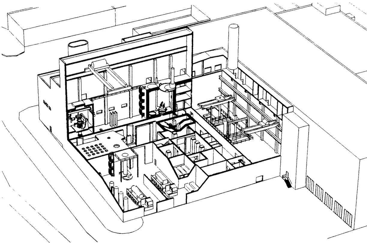
Figure 2.7          Encapsulation station for spent fuel.
