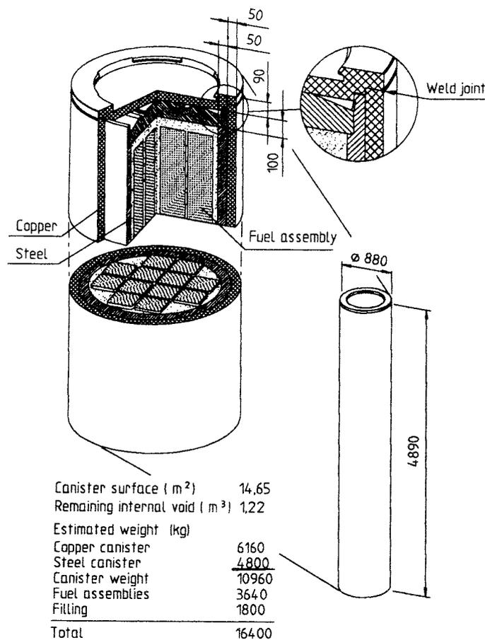
**Figure 2.6** Copper canister with an inner steel container
