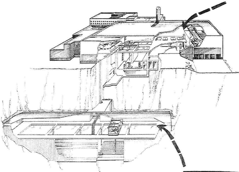
**The handling of storage canisters in the storage section**
