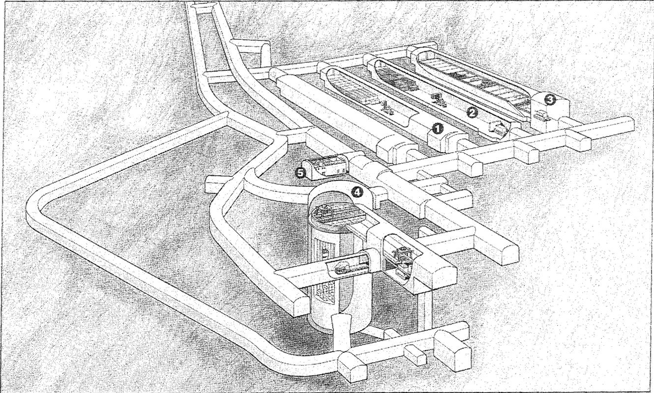
1. Rock vault for intermediate-level waste in concrete tanks. The tanks are handled by forklift truck.
