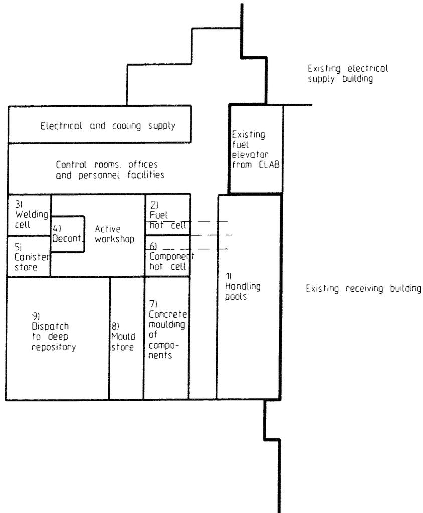
Figure A4.5 Key plan of the encapsulation plant
