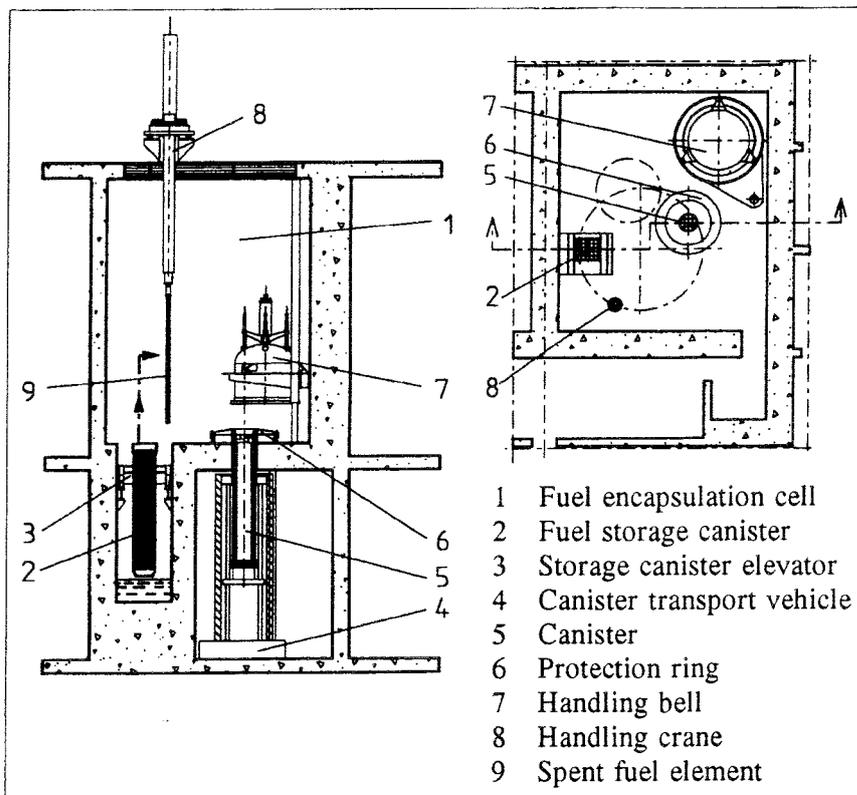
Figure A4.8 Hot cell for encapsulation of spent fuel
