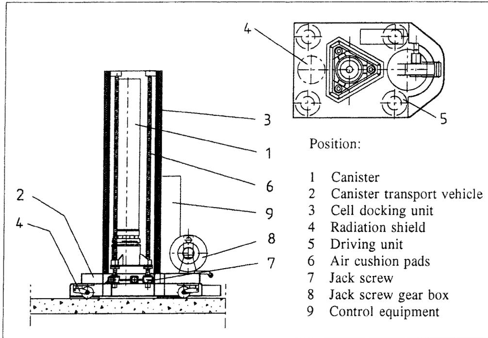
Figure A4.7 Copper canister with its radiation shield
