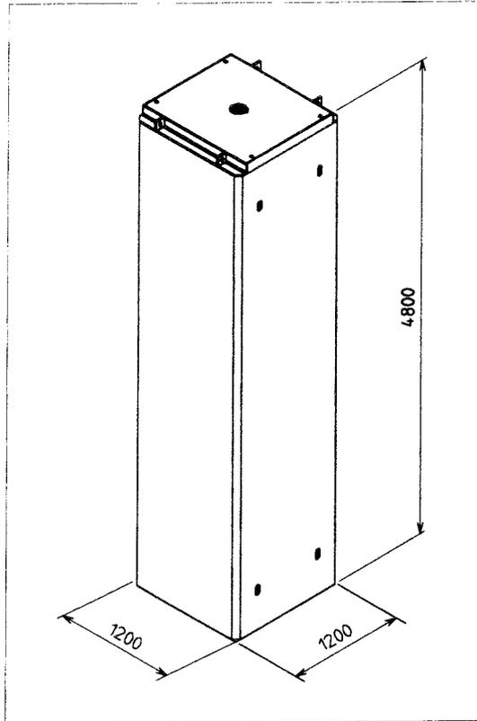
Figure A4.4 Concrete mould with core components.
