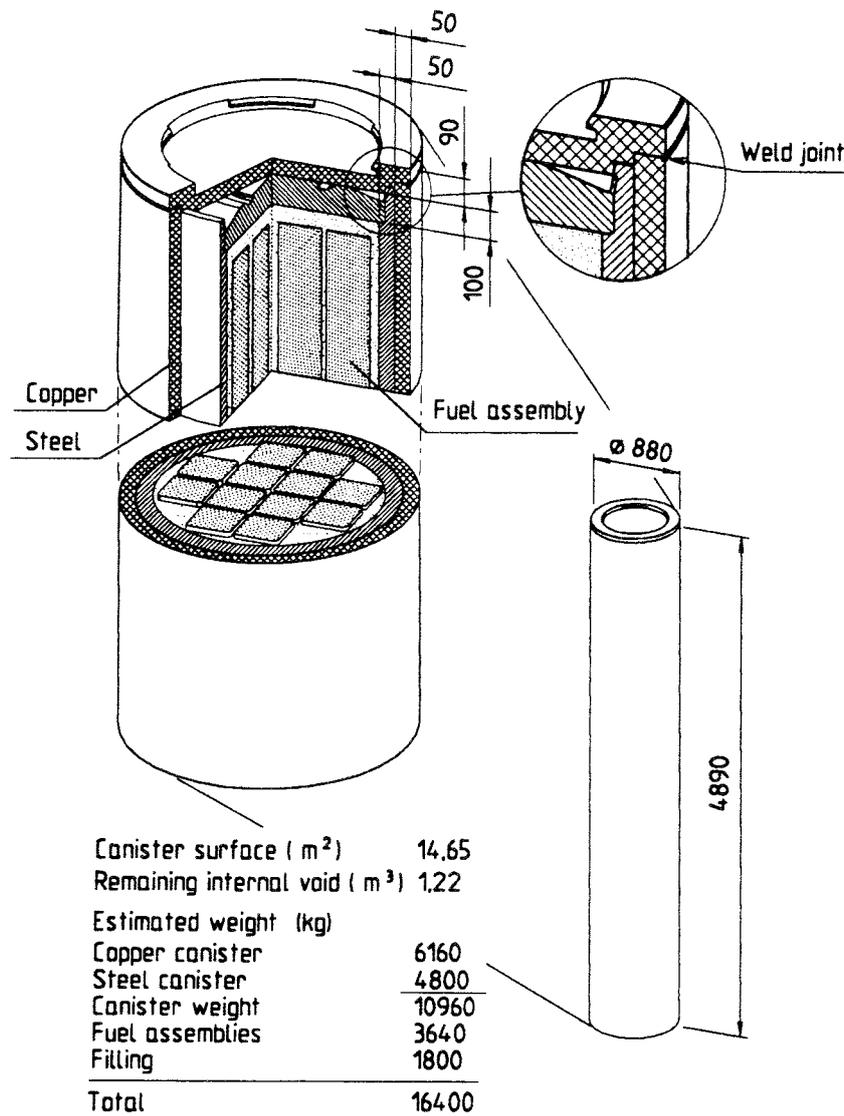
Figure A4.3 Canister with BWR-elements
