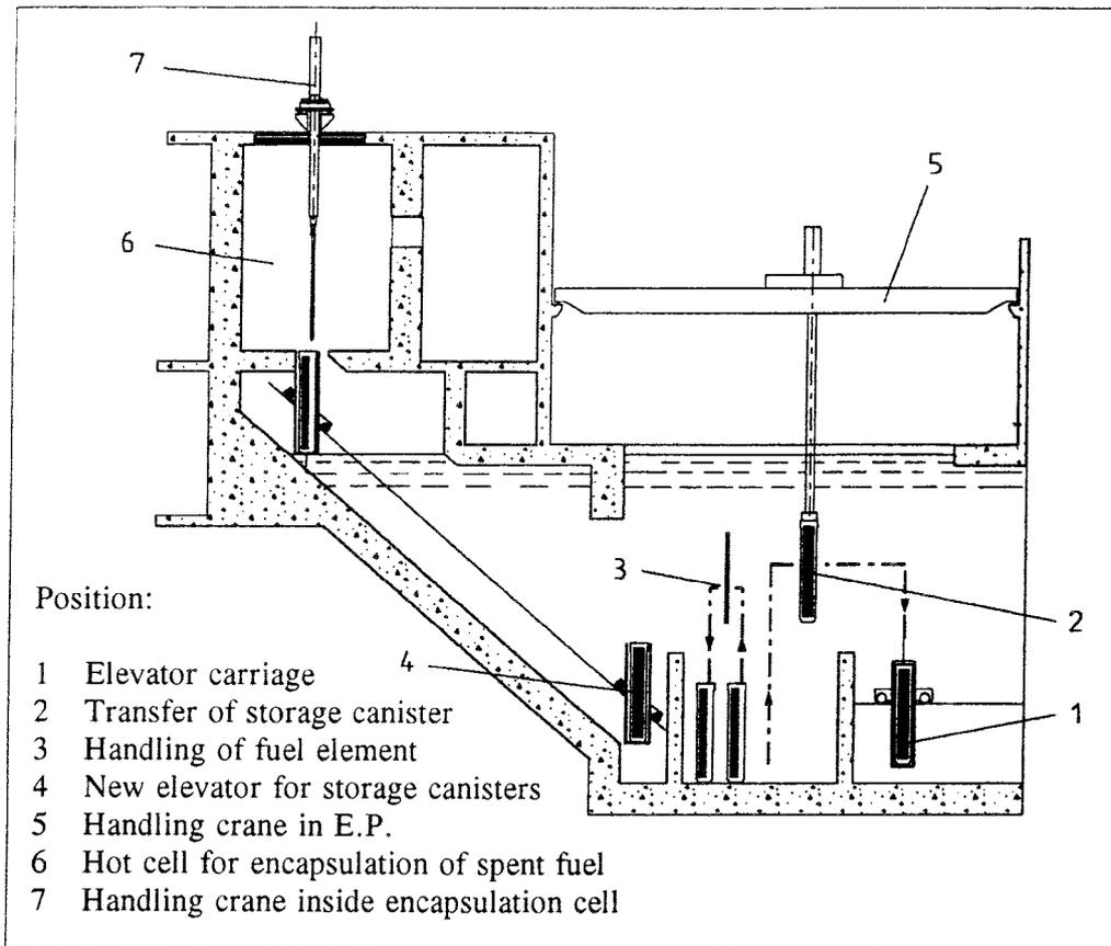
Figure A4.6 Handling pool and connection of a storage canister to the hot cell.
