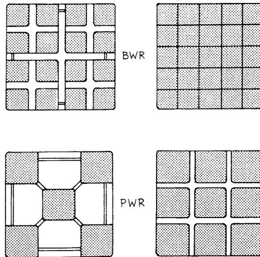
Figure A3.4 Design of the old and new canisters at CLAB.
