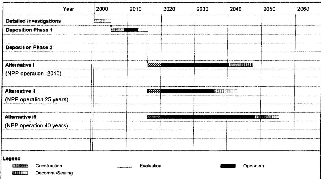
**Figure 3.1** Time schedule for deposition for different alternatives
