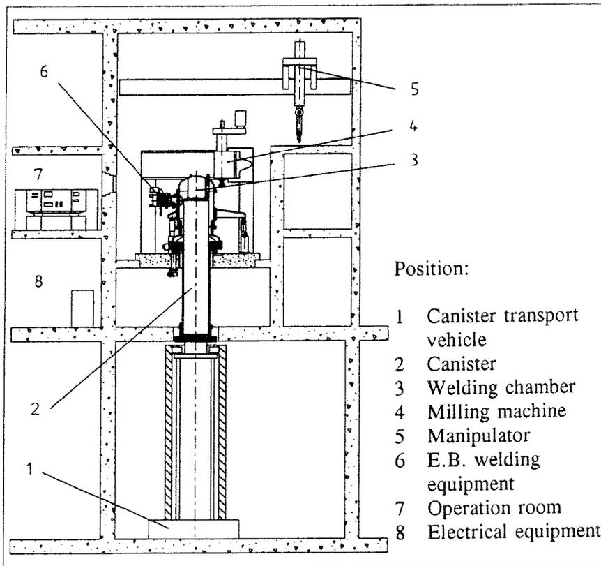
Figure A4.9 Welding and machining cell
