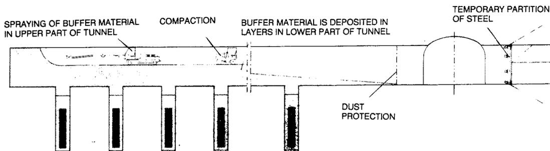
Figure A5.6 Backfilling of deposition tunnel
