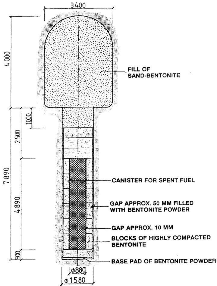
Figure A5.5 Deposition hole with canister and buffer material
