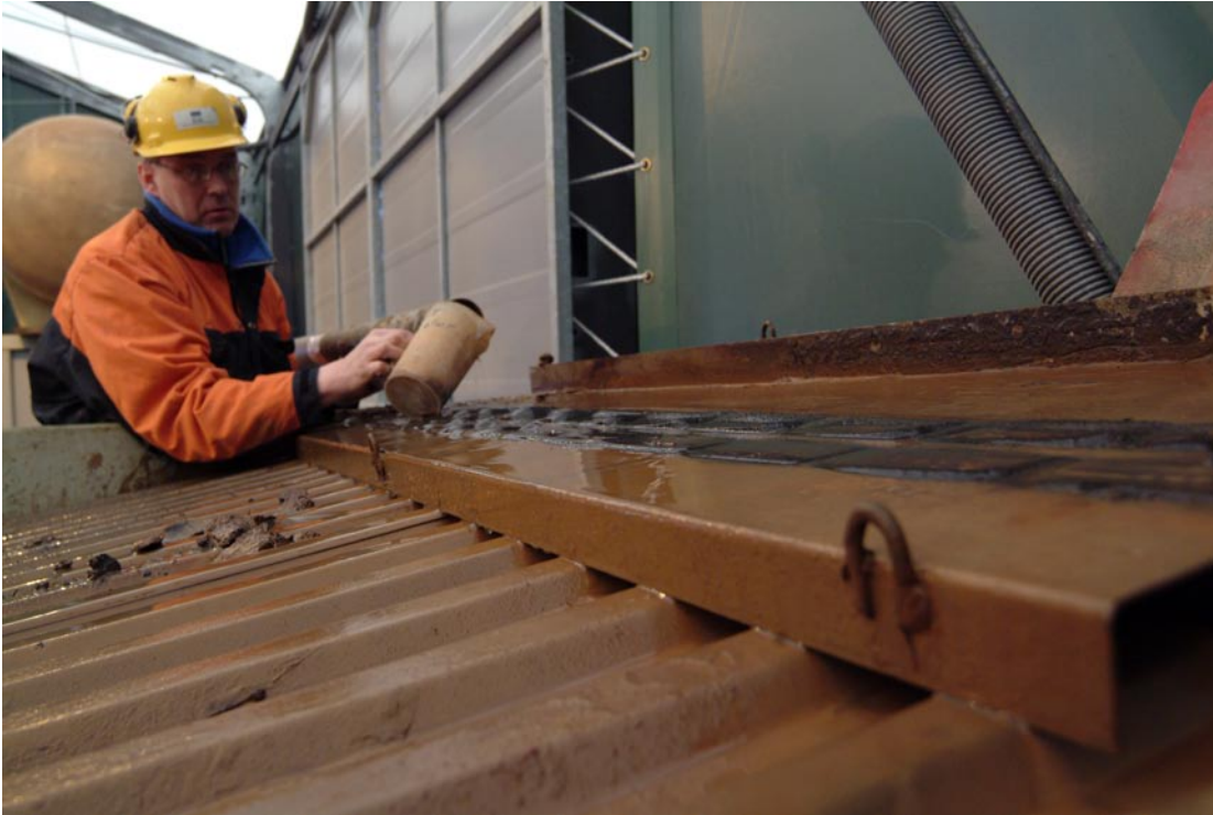
Figure 5-21. The outlet of return water pipe from the borehole is placed right above a magnetic steel plate mounted in the first container. Magnetic iron filings in the return water are caught on the plate during flooding of the return water over the plate. The filings are collected on a regular basis.
