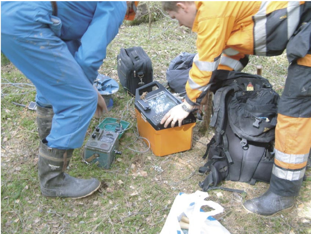
Figure 3-1. The recording instrument, ABEM Terraloc MK6.
