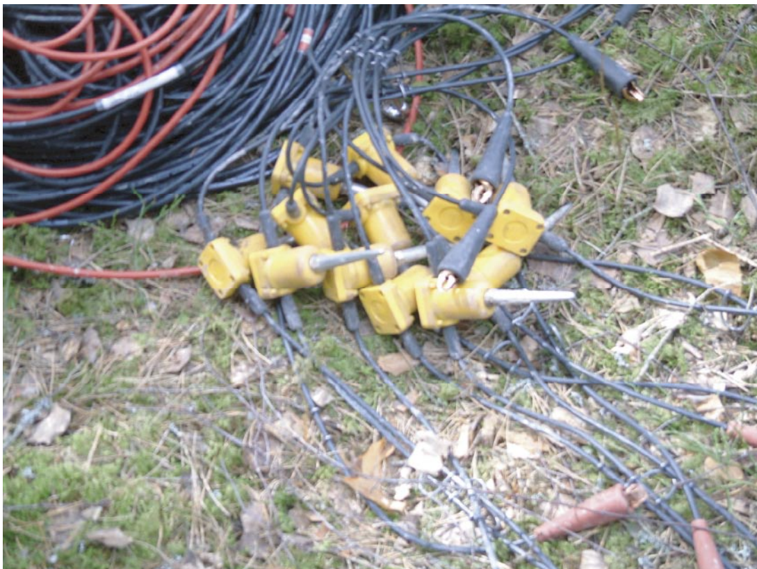
Figure 4-1. Geophones used during the survey.
