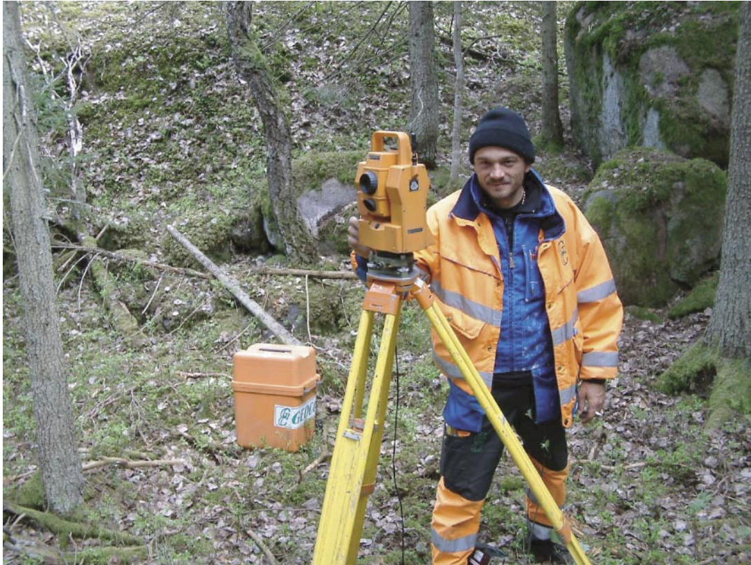
Figure 4-2. Line survey with Total station.
