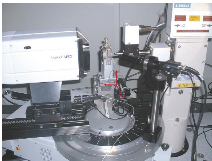
Figure 2-37. Set-up for micro-XRD used to determine the composition of the deposits from the bottom of the autoclave.
