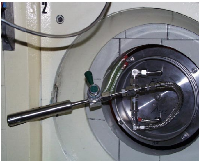
Figure 3-10. Gas collection cylinder outside the hot cell (volume 50 cm^3 ).
