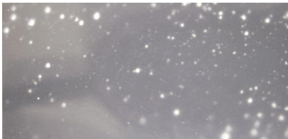
Figure 2-33. \alpha -autoradiography of the first irradiated CN85-film “UP”. The picture shows that most of the \alpha -activity is in form of U-particles. The U-particles have different grain sizes, proportional to the ^{233}\text{U} activity. U-particles located at some distance from the film give blunt spots.
