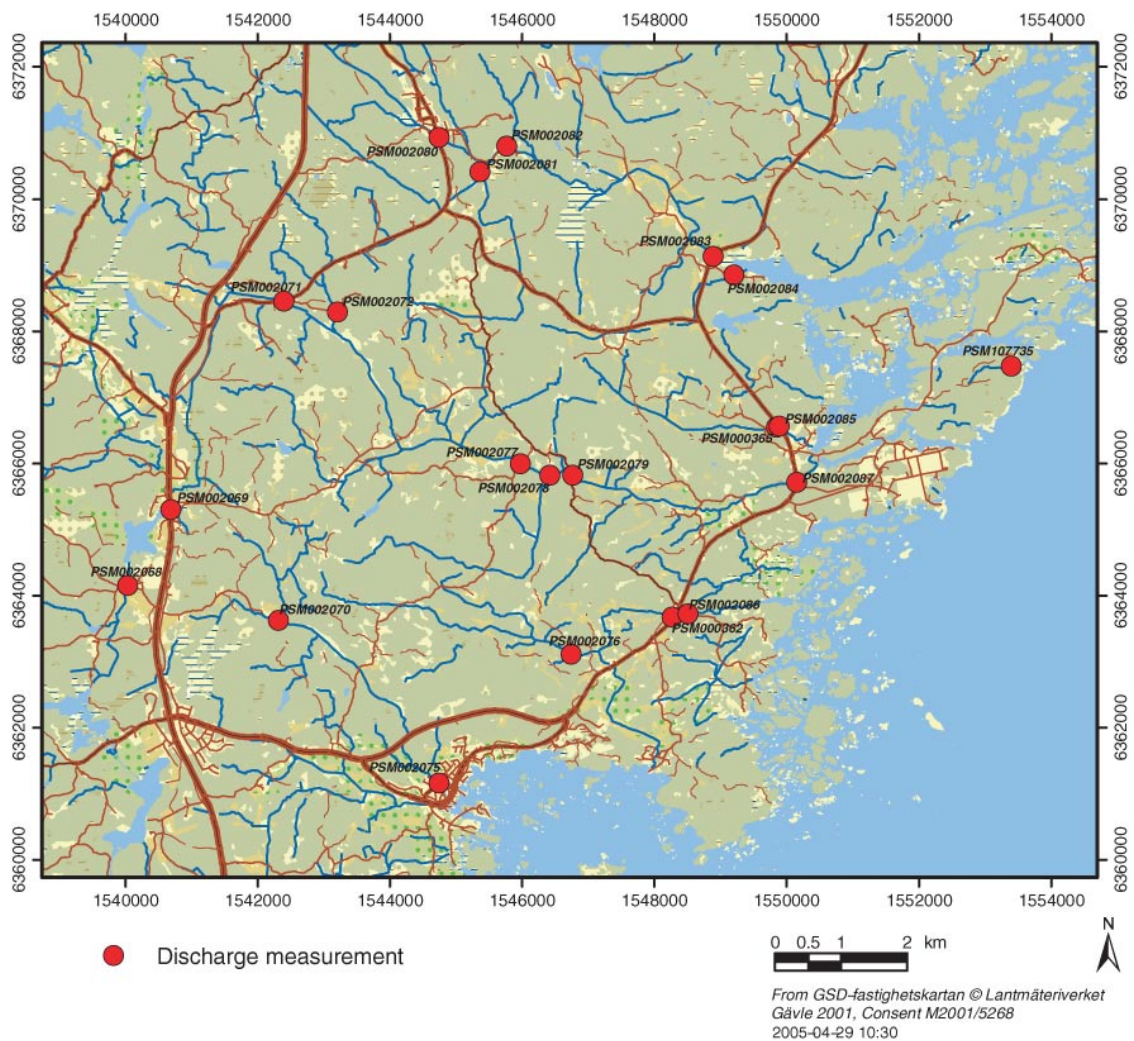
Figure 3-20. Map showing the locations of simple discharge measurements in water courses.
