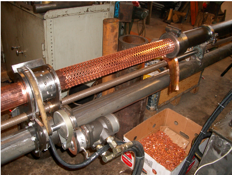
Figure 2-3 Manufactured perforated copper tube.
