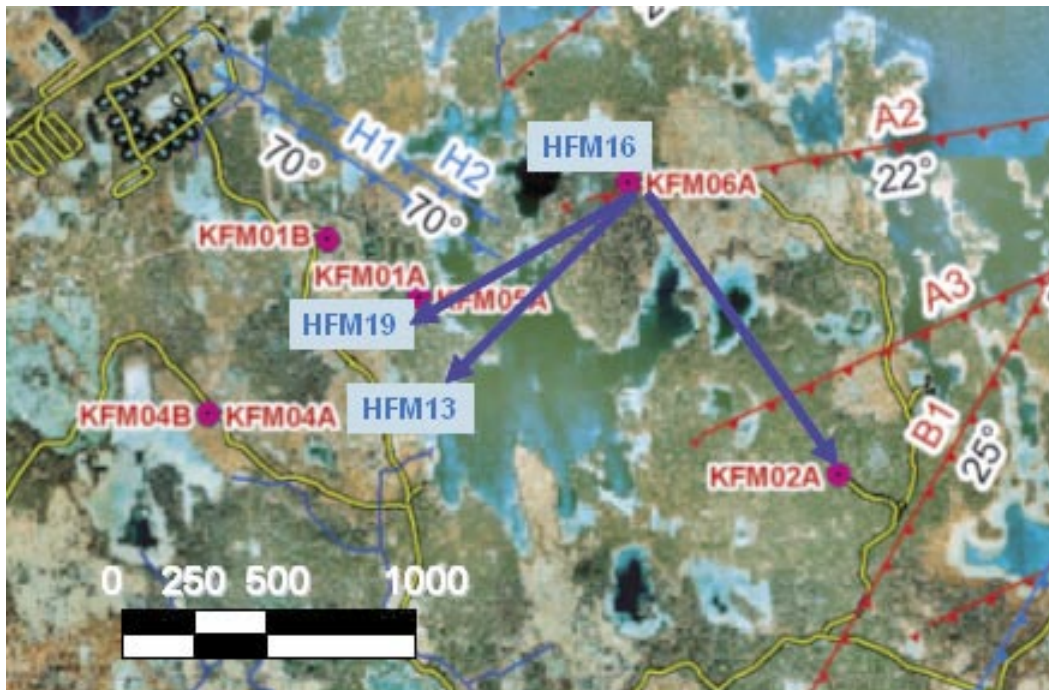
Figure 2-1. Key map showing the area around percussion borehole HFM16. Arrows indicate the assumed responding boreholes.
