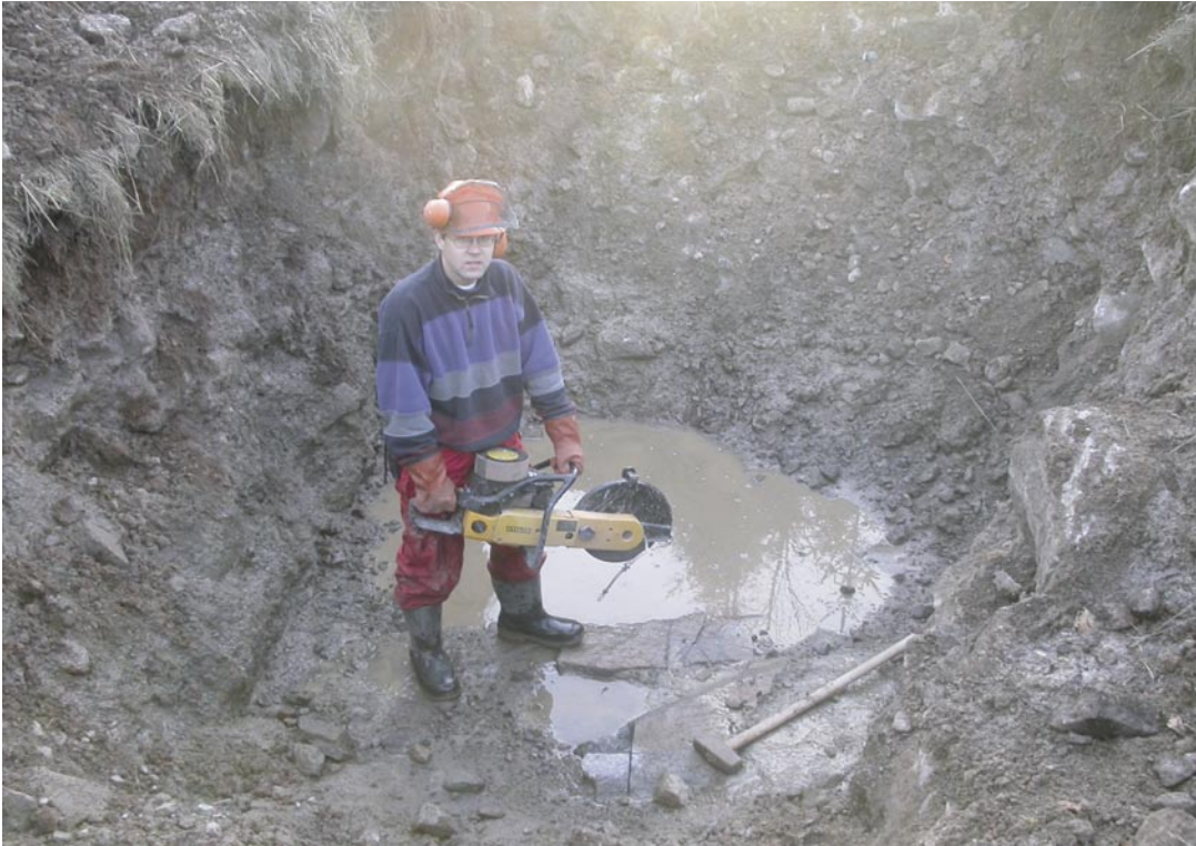
Figure 3-2. Torbjörn Bergman and the petrol-driven rock saw used for rock sampling.
