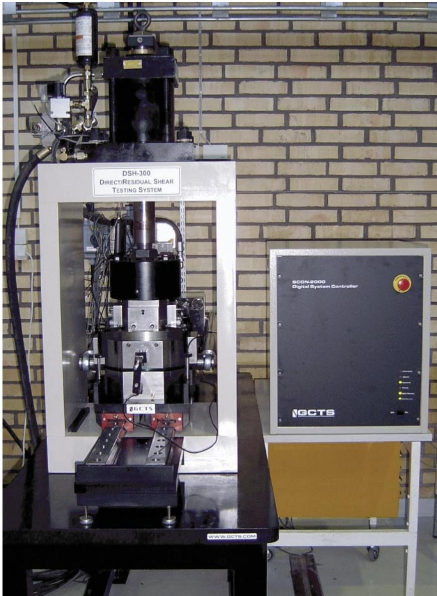
Figure 3-1. Equipment for direct shear tests, i.e. load frame and digital controller unit.
