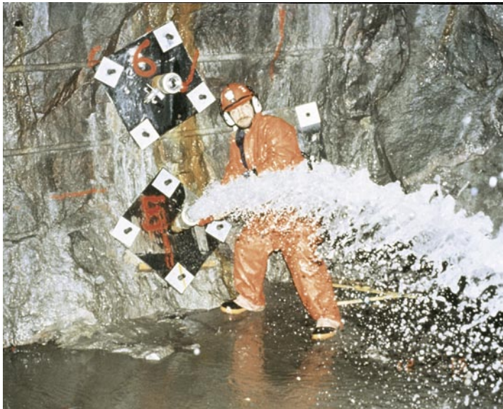
Figure A1-11. Extreme water pressures caused inflows of up to 1,350 l/min in certain drillholes /Rhén et al. 1993/.
