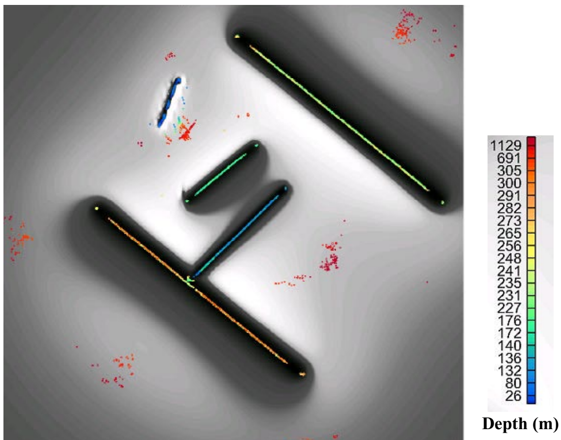
Figure 4-11. Solutions from the Euler deconvolution, SI = 1 (magnetic dyke), superimposed on the synthetic anomaly magnetic field. The background magnetic field is shown with an anti-grey colour scale.
