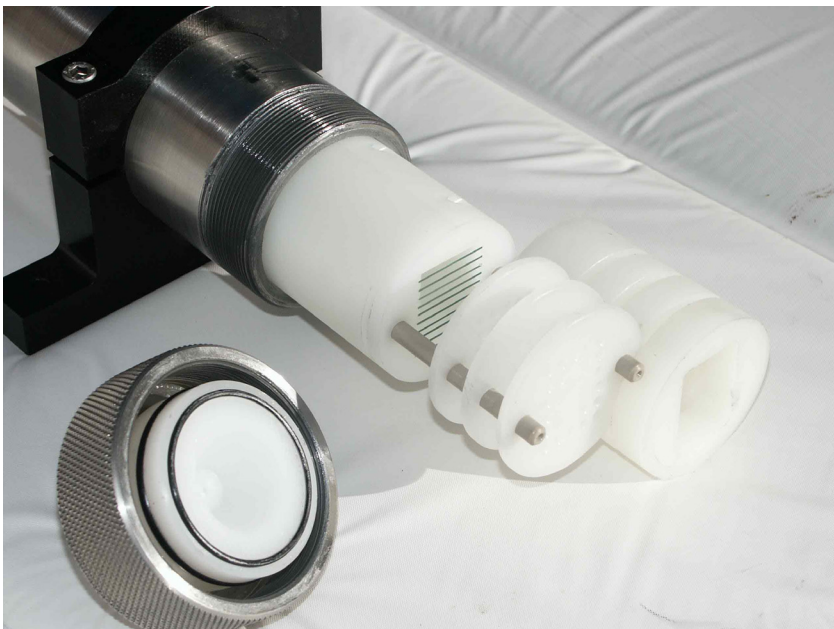
Figure 4-12 One of the twelve flow cells that are installed at the Microbe 450-m site is shown. Ten pieces of surfaces can be installed. They can be made of granite, glass metal or combinations, depending on the aim of the experiment. Three flow diffusers before and after the surface pile distributes the flow evenly over the test surfaces.
