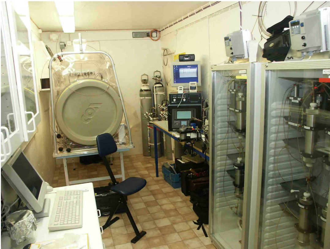
Figure 4-11. A view of the laboratory environment at the 450-m Microbe site is shown. The laboratory is equipped with three circulation systems (right), an anaerobic box (forward), an in situ gas extractor and a Kappa 5 gas chromatograph (right of the anaerobic box).
