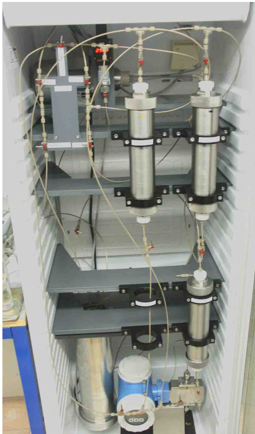
Figure 4-13 Left: Image of one of the three installed flow cell cabinets. (Lower left flow cell has been removed and sampled). Right: Schematic view of the cabinet.
