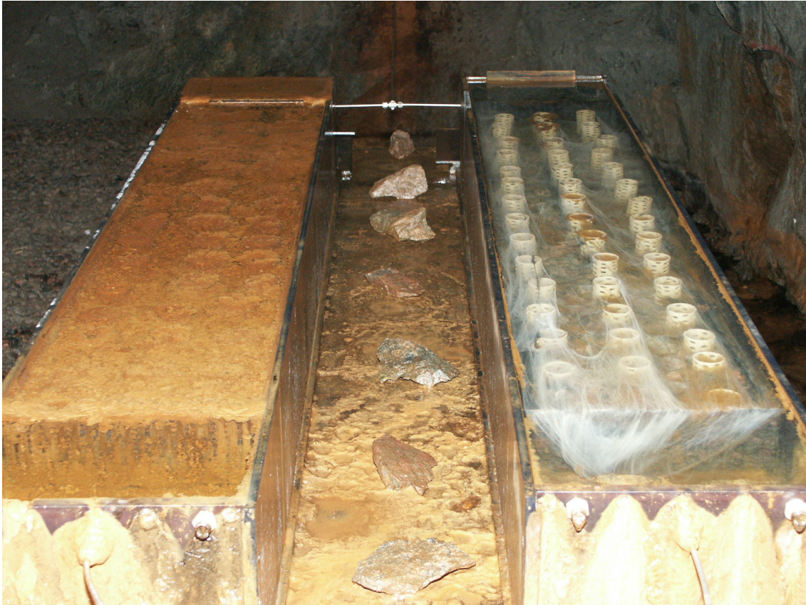
Figure 4-14 The artificial channels at 2,200-m Microbe site are feed by water from a common borehole, but they are inhabited by either iron oxidising microbes (left) or sulphur oxidising microbes (right). The balance between iron and sulphur microbes is very delicate. A small difference in the inlet profile of ground water results in a huge difference in the structure of the respective population.
