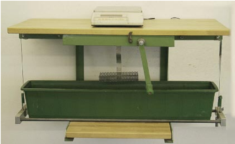
Figure 3-1. Experimental set-up for density measurements by the buoyancy method.
