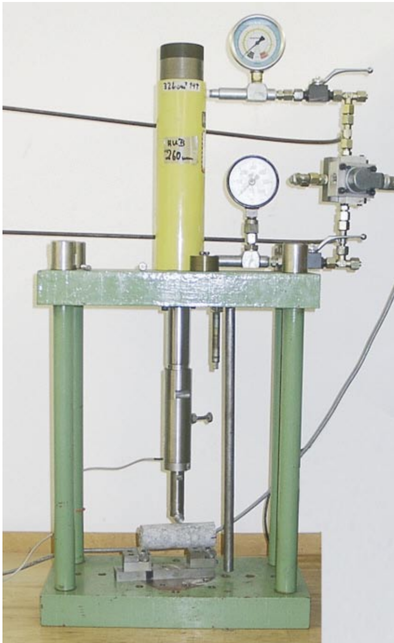
Figure 3-5. Experimental set-up for fracture toughness testing.
