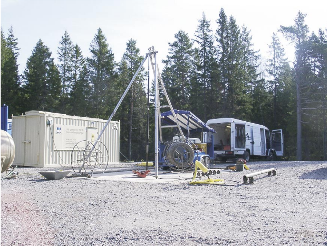
Figure 3-2. Photo showing the wireline hydrofrac system at the location of borehole no KFM02A.
