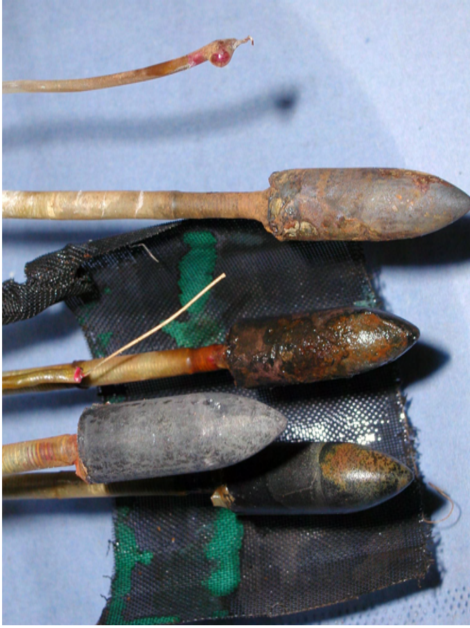
Figure 36. Specimens at end of Test 6 (deaerated Allard water at 50° C, left Cell A, right Cell B)
