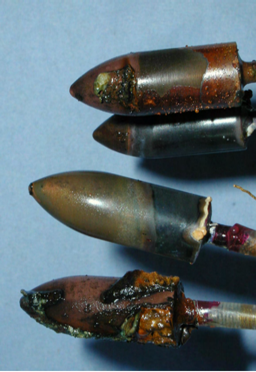
Figure 9. Specimens at the end of Test 1 (deaerated bentonite-equilibrated groundwater at 30° C).
