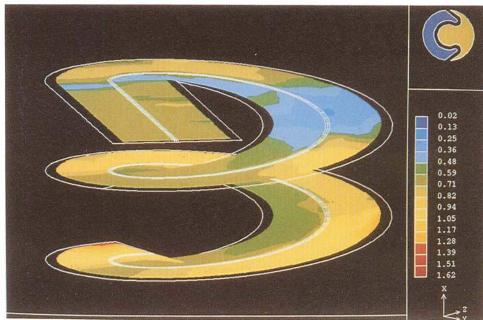
Figure 5-12. Estimated salinity of groundwater seeping into the tunnel after blasting to full depth (steady-state phase).
