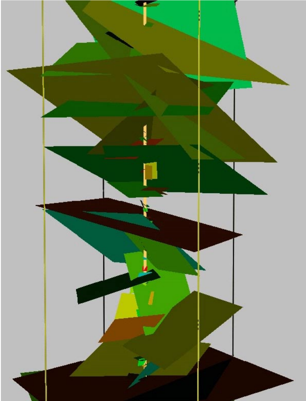
Figure 3-35. Close-up of fractures intersected by borehole KSH01A to show different scales of fractures seen in borehole. Fractures are coloured by \log(T) (in this case T is lognormally distributed and not correlated to L ).
