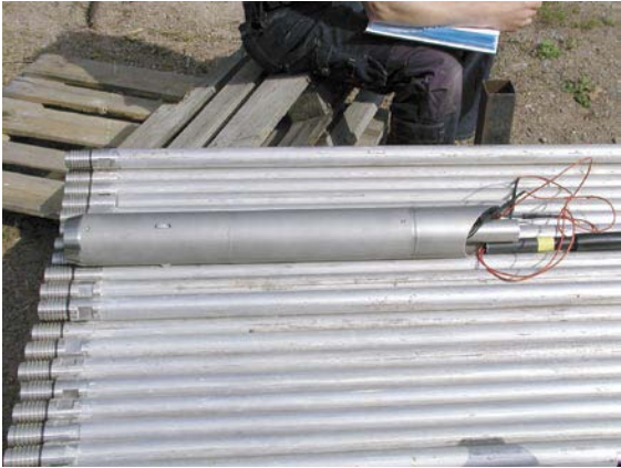
Photo 5. Positioner, bottom end of down-hole string.
