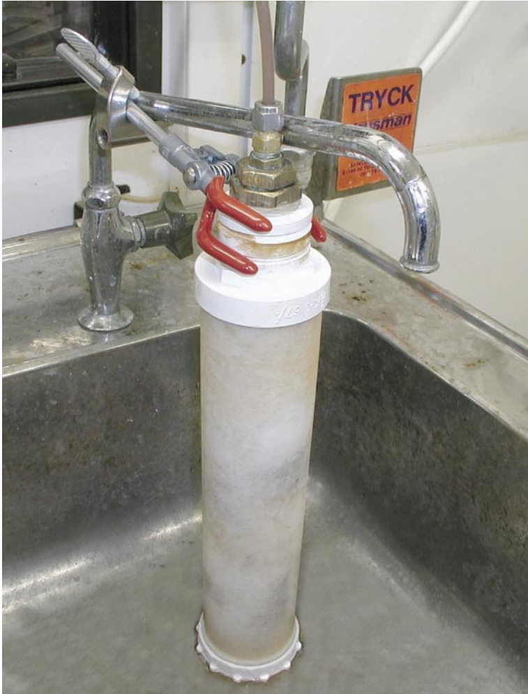
Figure 3-3. Water from the borehole passes through the ion exchanger in the column.
