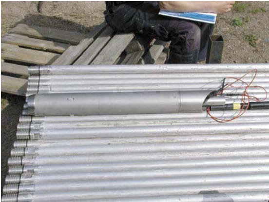
Photo 5. Positioner, bottom end of down-in-hole string.
