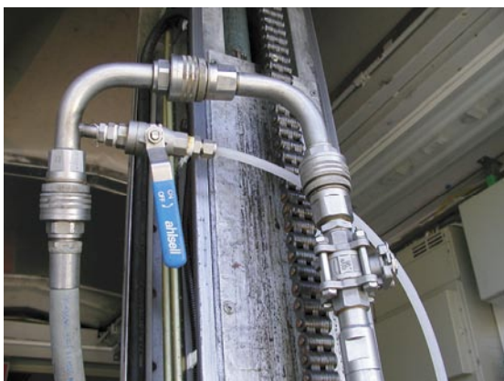
Photo 5. Top of test string with shunt valve and nylon line down to the pump basket.
