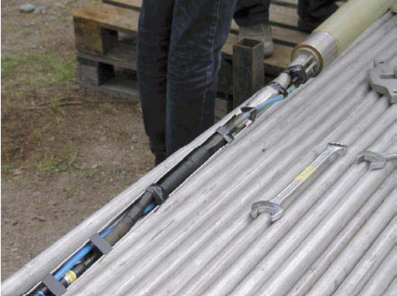
Photo 4. Pressure vessels for test valve, packers and injection.
