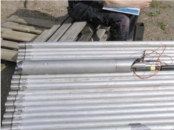
Photo 5. Positioner, bottom end of down-hole string.
