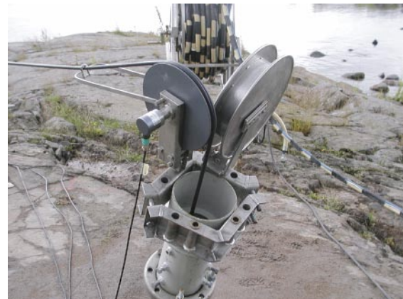
Photo 4. Depth measuring wheel on TOC.
