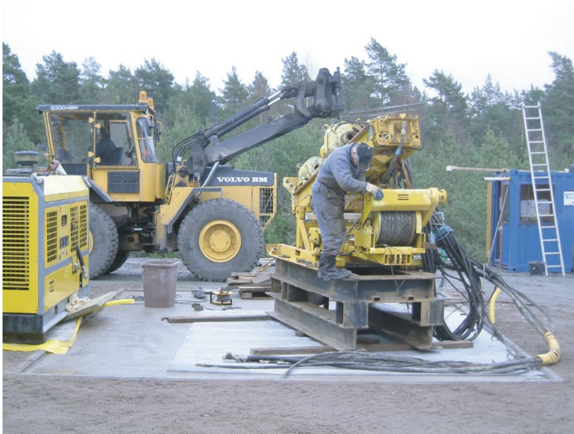
Figure 4-1. Establishing the drill rig at the KAV04 drill site.
