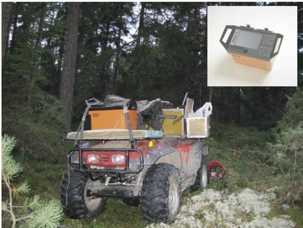
Figure 3-1. The seismic equipment (ABEM Terraloc MK6, also shown on inserted picture) mounted on a small field truck.
