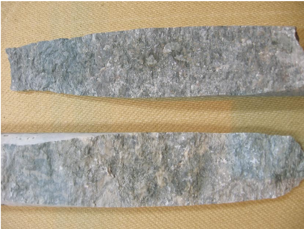
Figure 4-1. Upper and lower joint surfaces used in the tilt test apparatus.
