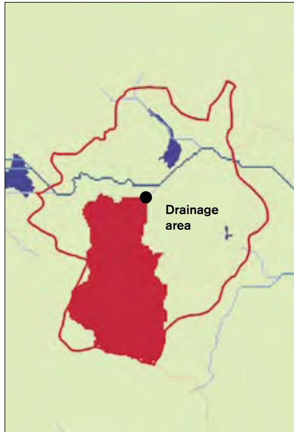
Figure C-12. The area upstream (red) the discharge point (black dot) is multiplied with area specific runoff to obtain the waterflow at the discharge point.
