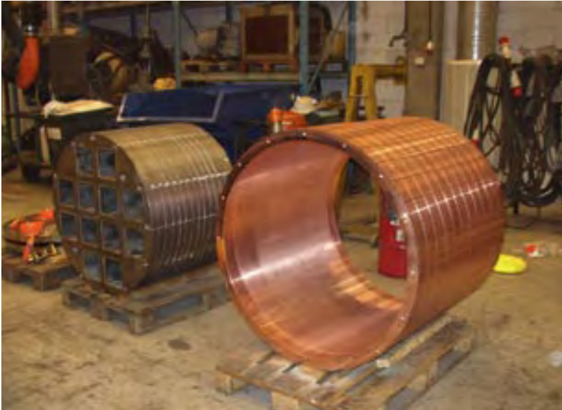
Figure 6-1. Part of cast iron insert and copper canister for pressure test.
