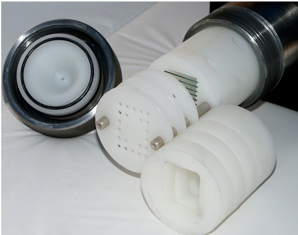
Figure 2-11. The pressure-resistant flow cell with a shell of stainless steel. The interior is made of a polymer material called polyvinylidene fluoride (PVDF). Three flow diffusers distribute the flow evenly over all test surfaces in the test pile. The steel is not in contact with the groundwater.
