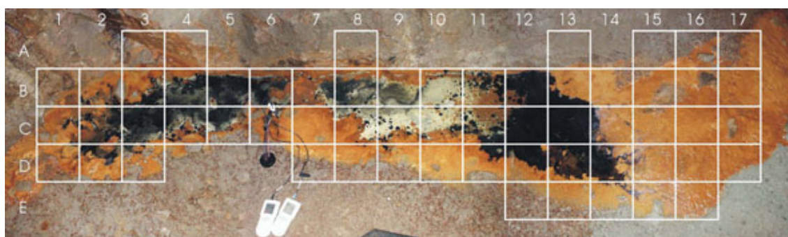
Figure 2-2. The 907-m ditch site is located at a depth of about 130 m and is characterized by a shallow, elongated pond that overflows into the main tunnel ditch to the right in the image. The brown material is BIOS. The black colour results from iron sulphide precipitates and the white material is calcium carbonate. The overlaid grid created an organized environment and enabled pH, oxygen, and redox measurements to be made in three dimensions. Field instruments are shown at the bottom of the figure. Grid size is about 20 × 20 cm.
