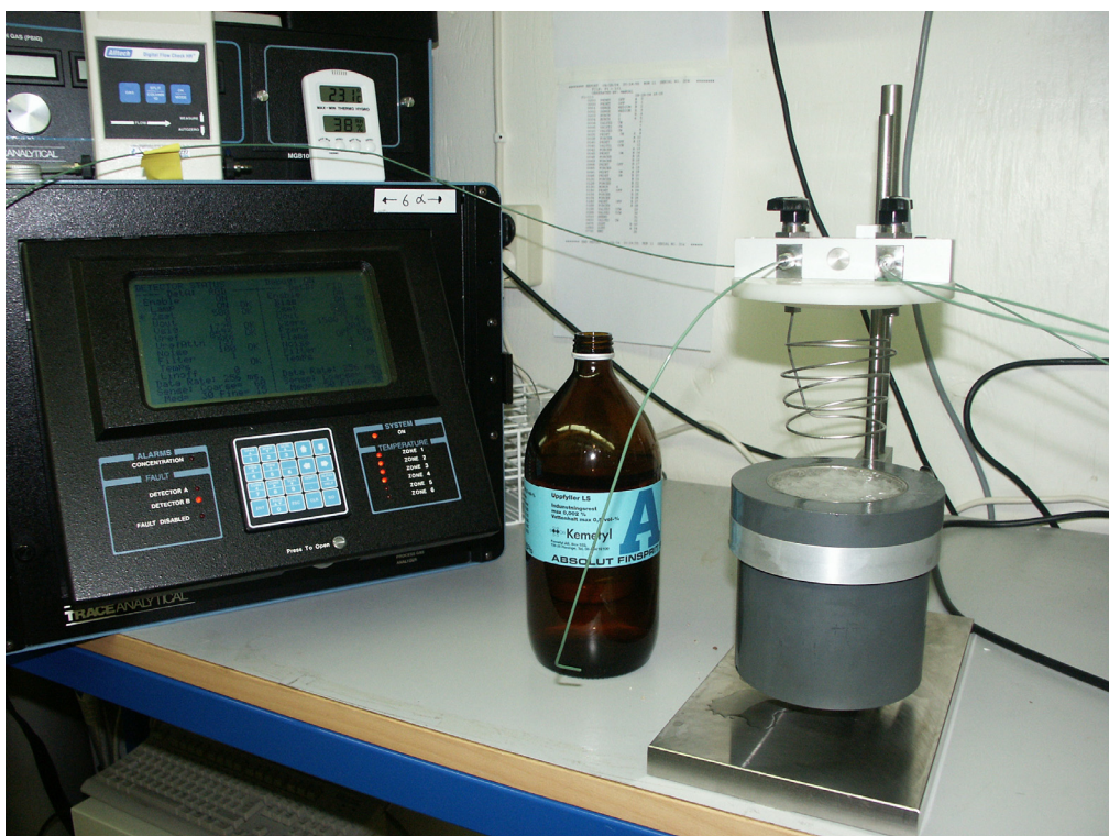
Figure 2-14. The on-line cryo trap with CO 2 pellets mixed with 99% ethanol for removing moisture from gas extracted from groundwater.
