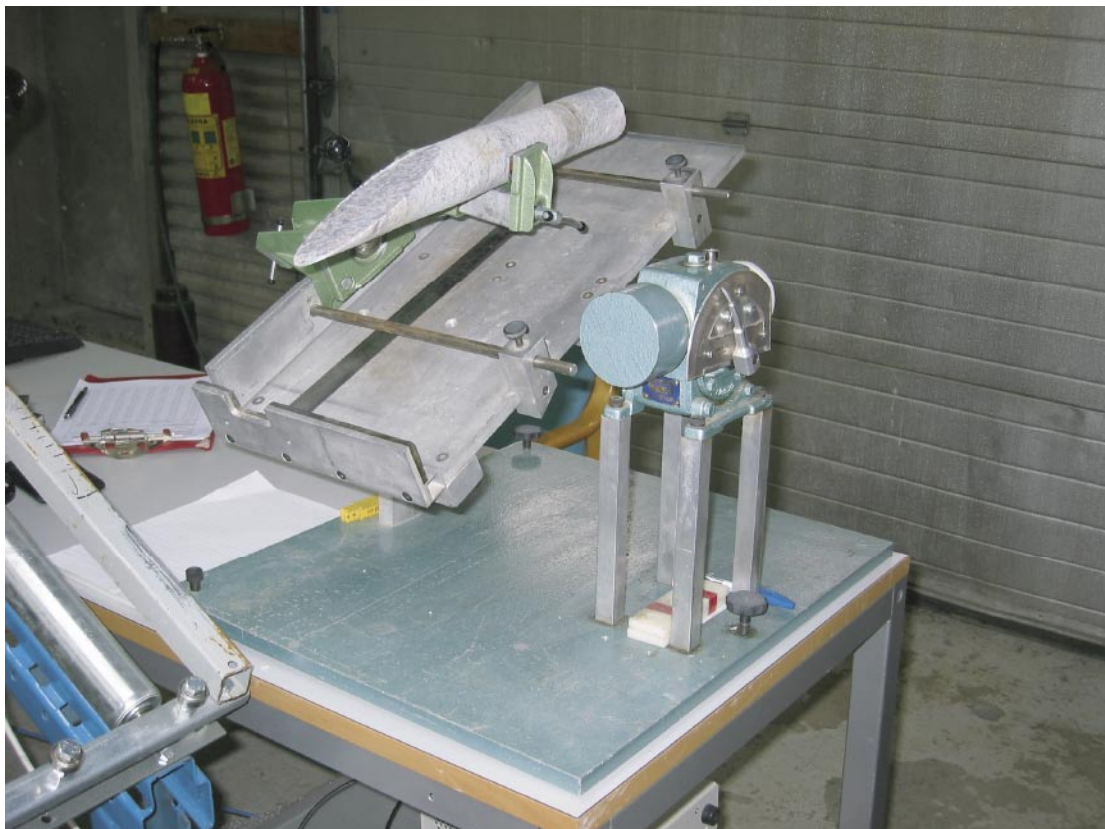
Figure 3-1. NGI's tilt test apparatus.
