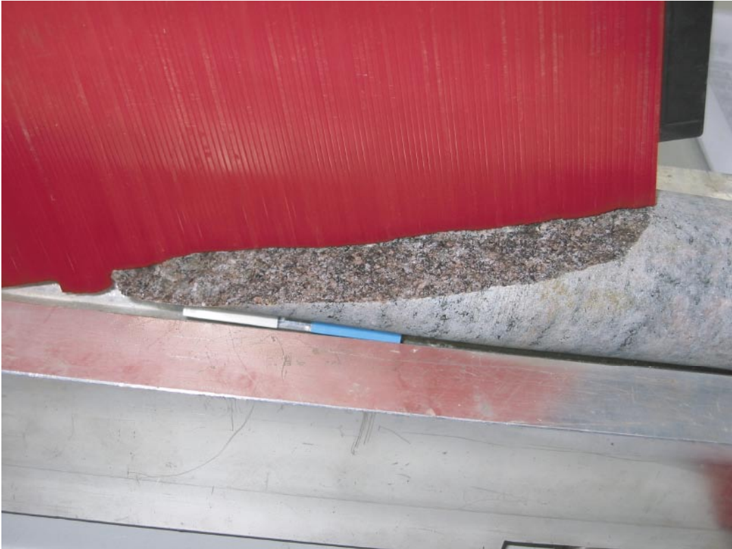
Figure 3-3. Profilometer applied on a joint surface.
