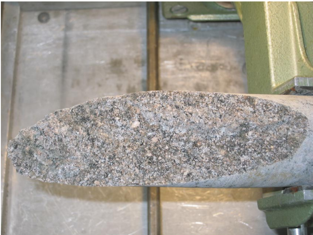
Figure 4-1. Single joint surface for the tilt testing.
