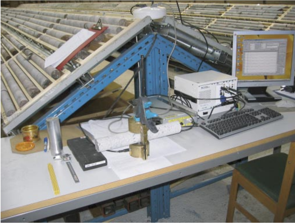
Figure 3-2. NGI's equipment set-up for measuring acoustic P-wave travel time transverse the drill core.
