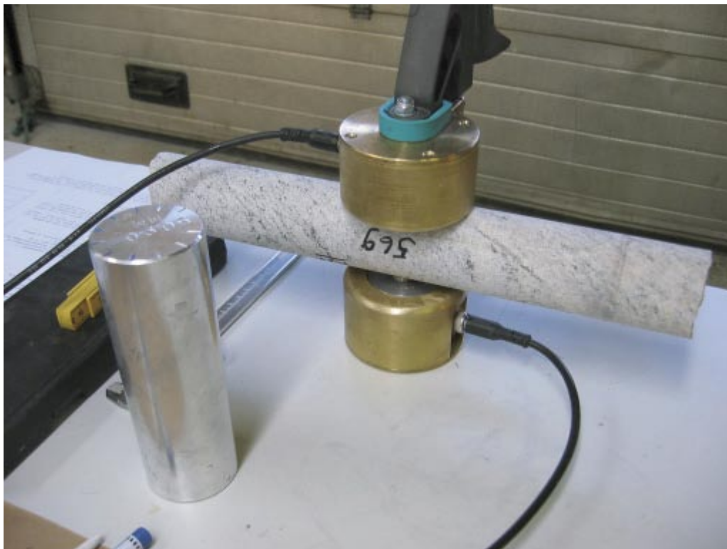
Figure 3-1. Detail of NGI's apparatus for measuring acoustic P-wave travel time transverse the drill core. The aluminium cylinder for calibration of the device is on the left.
