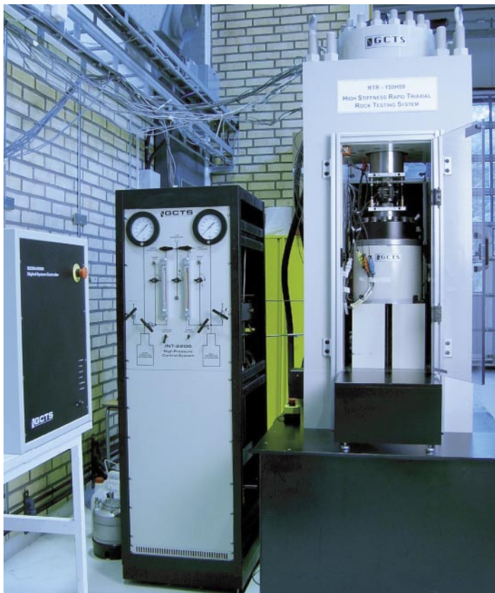
Figure 3-1. Rock testing system. From left: Digital controller unit, pressure cabinet (used for triaxial tests) and load frame. The PC with the test software (not shown in the picture) is placed on the left hand side of the controller unit.
