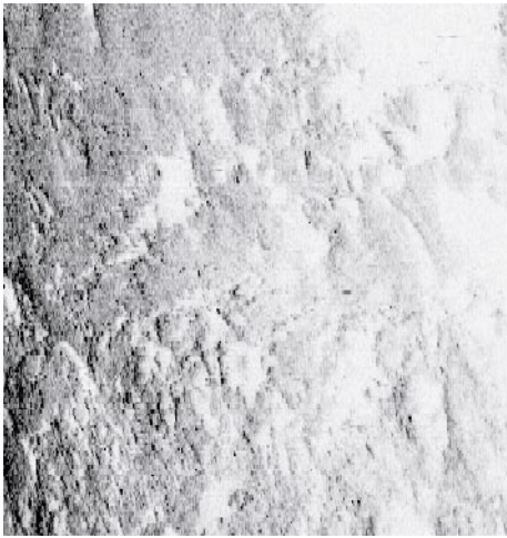
Figure 6-3. Sonar image of exposed bedrock.
