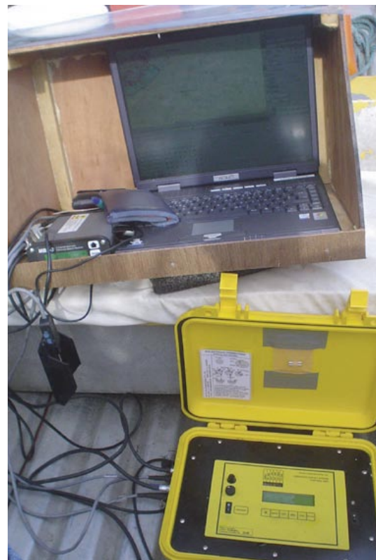
Figure 4-2. (Right) Navigation computer and top unit of the ceeducer single beam echo sounder used on the shallow survey vessel.
