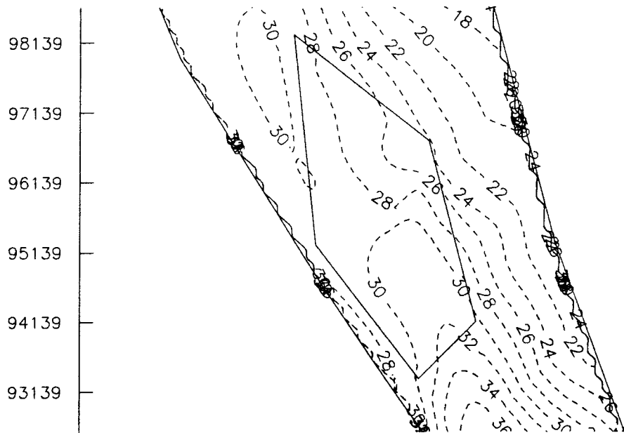
Figure 7.4a Blow-up of the pressure distribution at a level of z=-200 m; Case 3DSB, the Base Case on the semi-regional scale.
