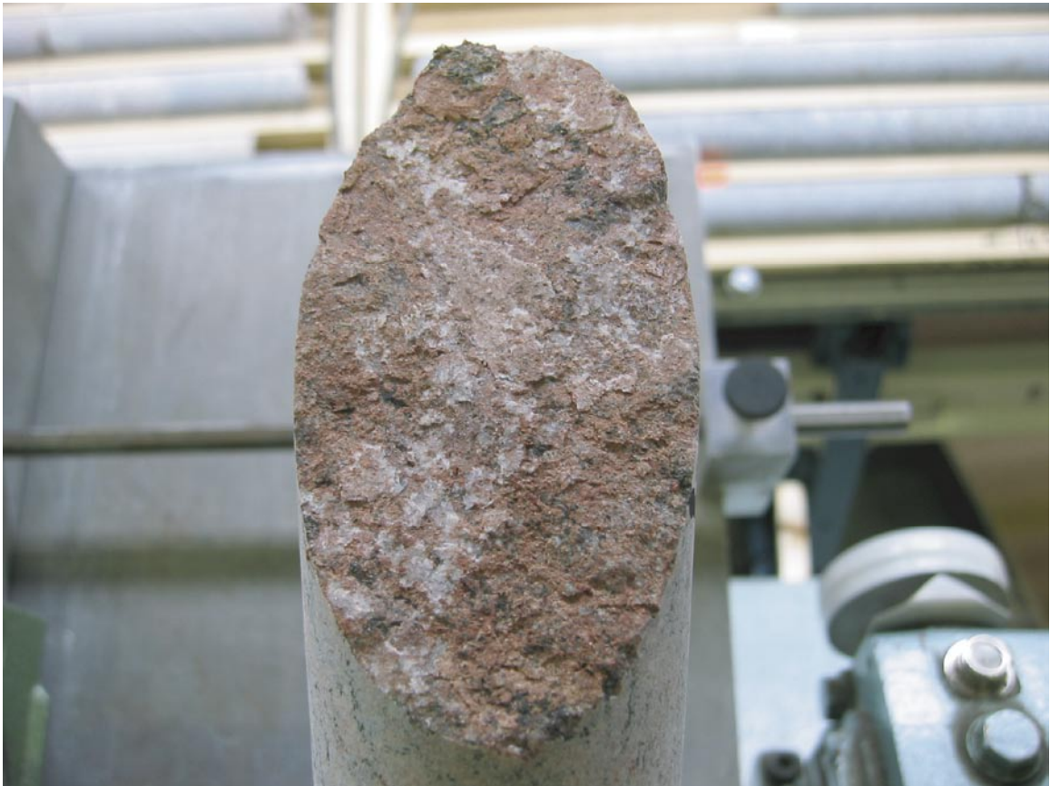
Figure 4-1. Lower joint surface of a core sample at test position in the tilt test apparatus.
