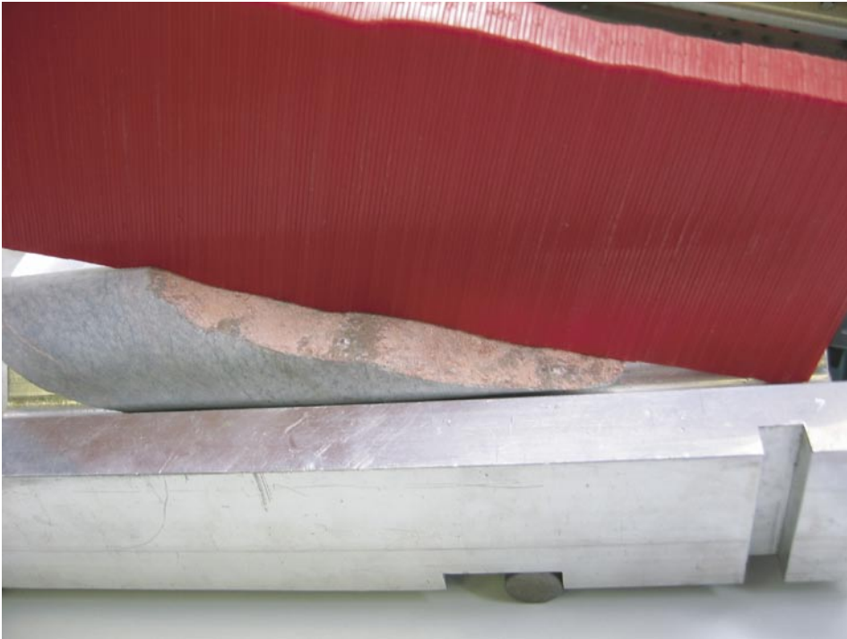
Figure 3-3. Profilometer applied on a joint surface.
