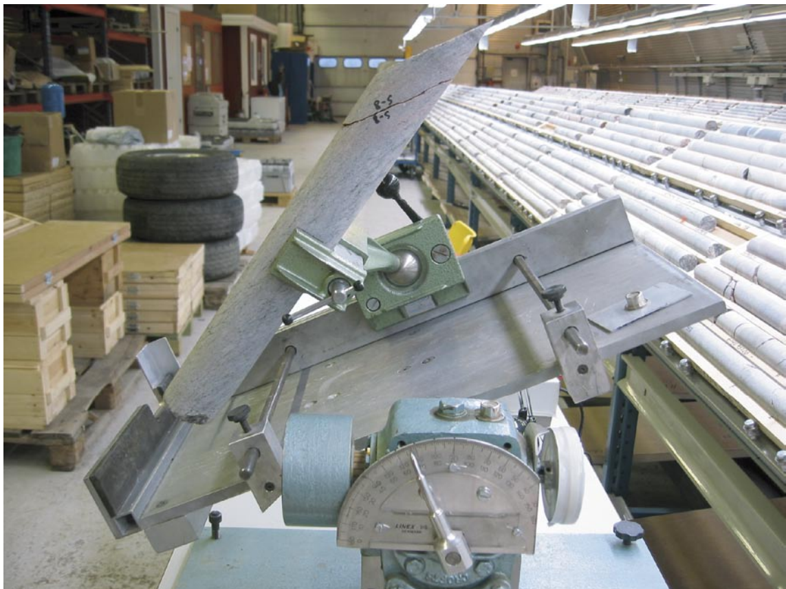
Figure 3-1. NGI's tilt test apparatus.
