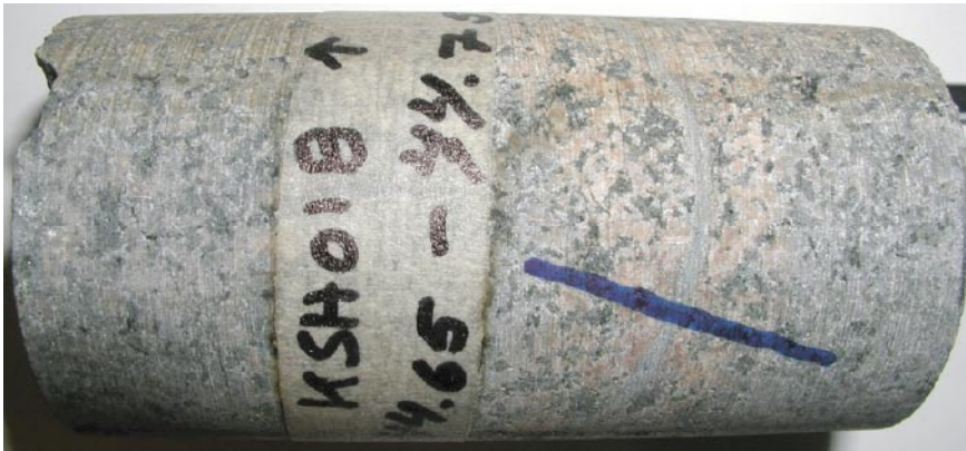
Figure 8-19. Photograph of the drill-core sample from 44.65–44.75 m, showing red-staining of the wall-rock adjacent to a prehnite filled fracture. Drill-core is 5 cm in diameter.
