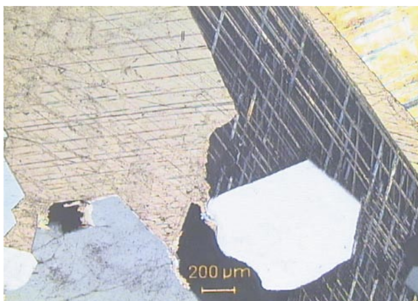
Figure 8-2. Idiomorphic quartz crystals and calcite crystals. Photomicrograph from thin-section KSH01 873 m.
