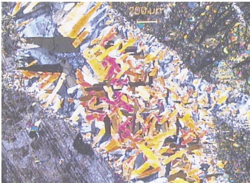
Figure 8-5. Idiomorphic prehnite filling a fracture that is penetrating through earlier formed epidote mylonite (upper right). Microphotograph from thin-section KSH01: 11 m.
