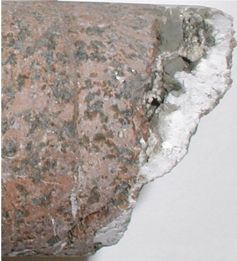
Figure A-6. Photo of the drill-core, showing the open fracture with big calcite crystals. Drill-core diameter is 50 mm.
