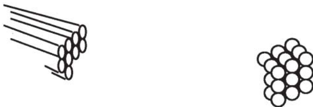
Figure 3-31. The timber pile structure of the 2D case and the ball case in 3D naturally give quite different void geometries.
