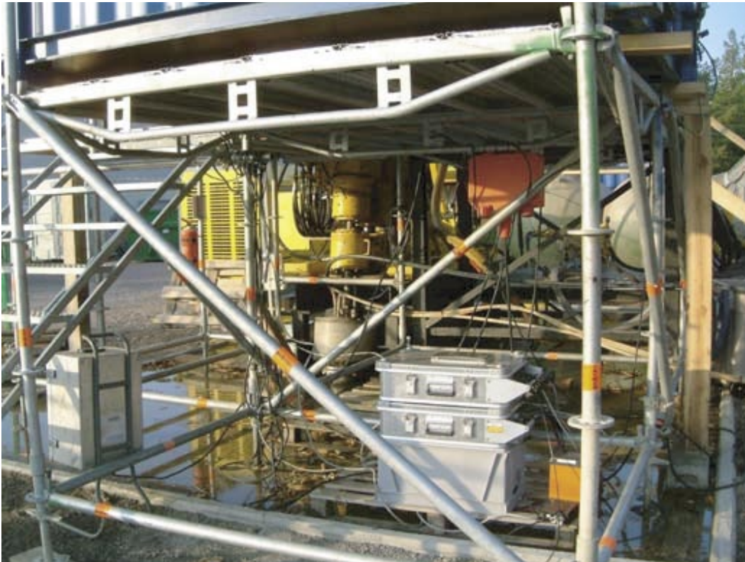
Figure 4-4. The CR23 logging unit for parameters “air-pressure” and “electrical conductivity”.
