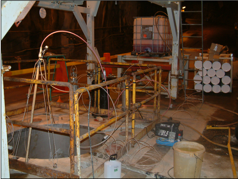
Figure 3-32. The Lasgit hole, the coloured water test. One of the anchor holes with a packer inserted (to the left), the empty Lasgit hole and in the background the container with Rhodamine WT coloured water.
