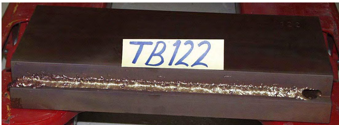
Figure 6-6. Weld TB 122. Welding test with oscillating beam.
