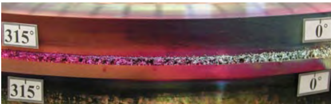
Figure 6-10. Lid weld L028. Section welded without oscillating beam.
