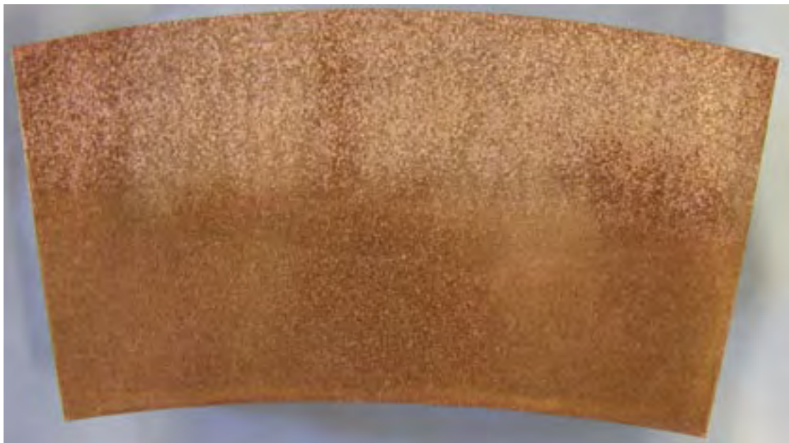
Figure 6-13. Lid weld L026. Longitudinal section in weld, length approximately 200 millimetres. The coarse structure shows the penetration of the weld.
