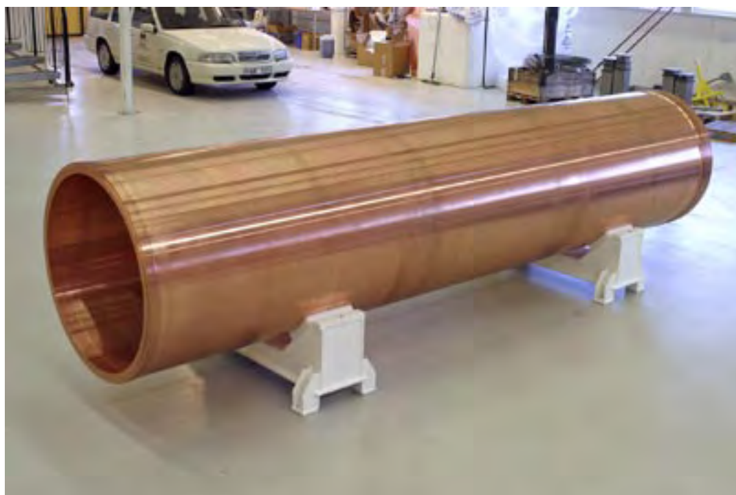
Figure 5-11. Extruded and machined copper tube.
