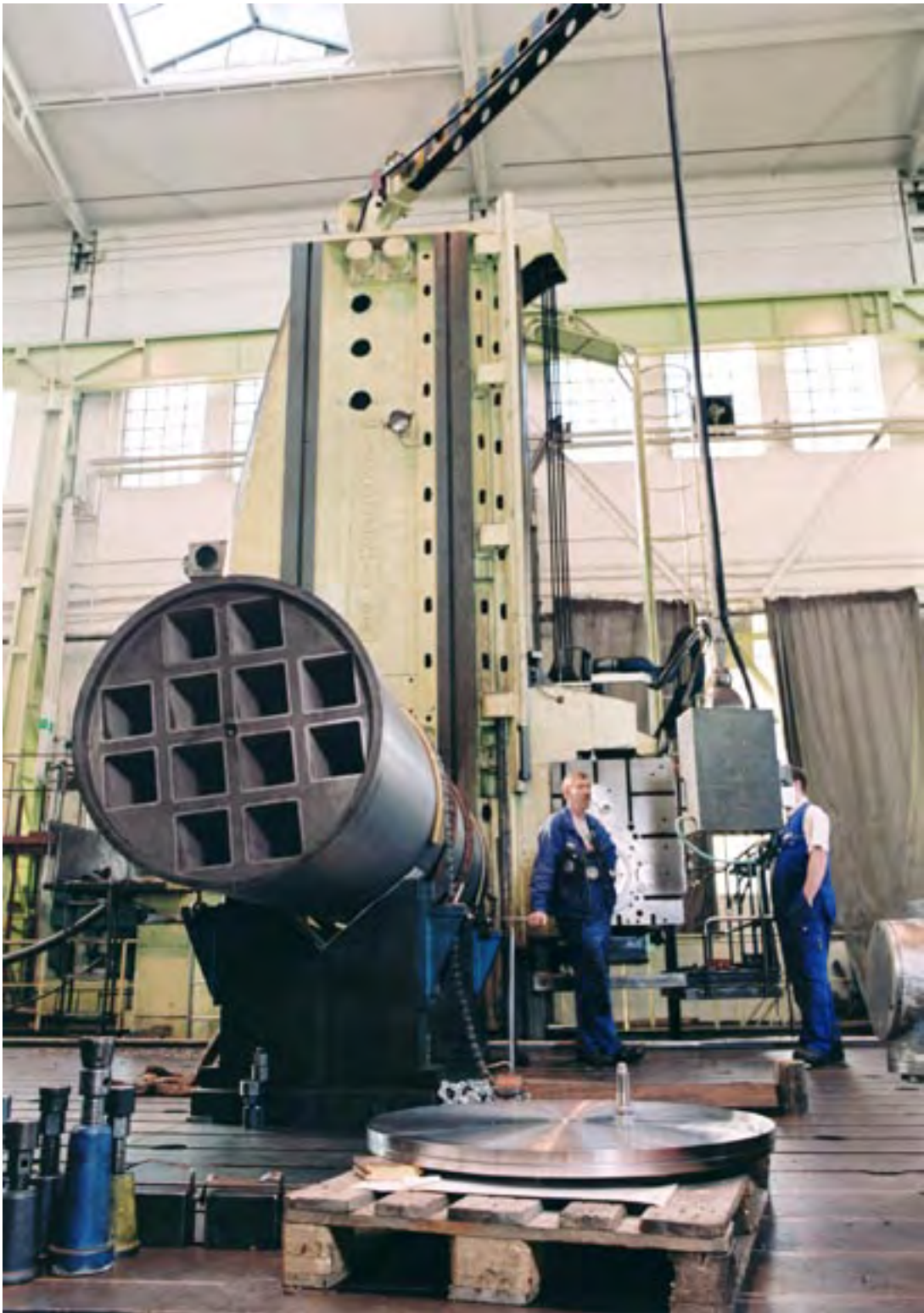
Figure 5-10. Finish-machined insert and steel lid for insert.
