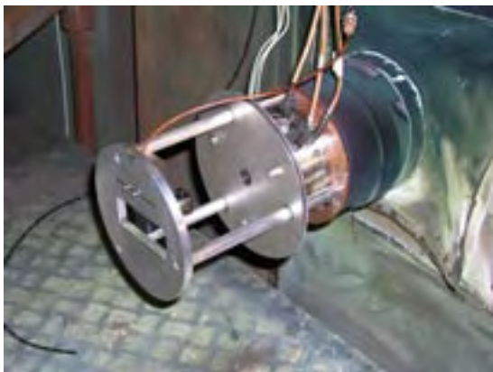
Figure 6-3. Coil with holder for beam deflection.
