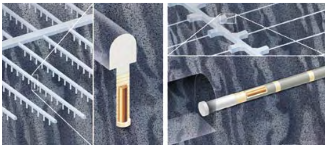
Figure 10-5. Fundamental difference between the reference method KBS-3V (left) and KBS-3H (right).
