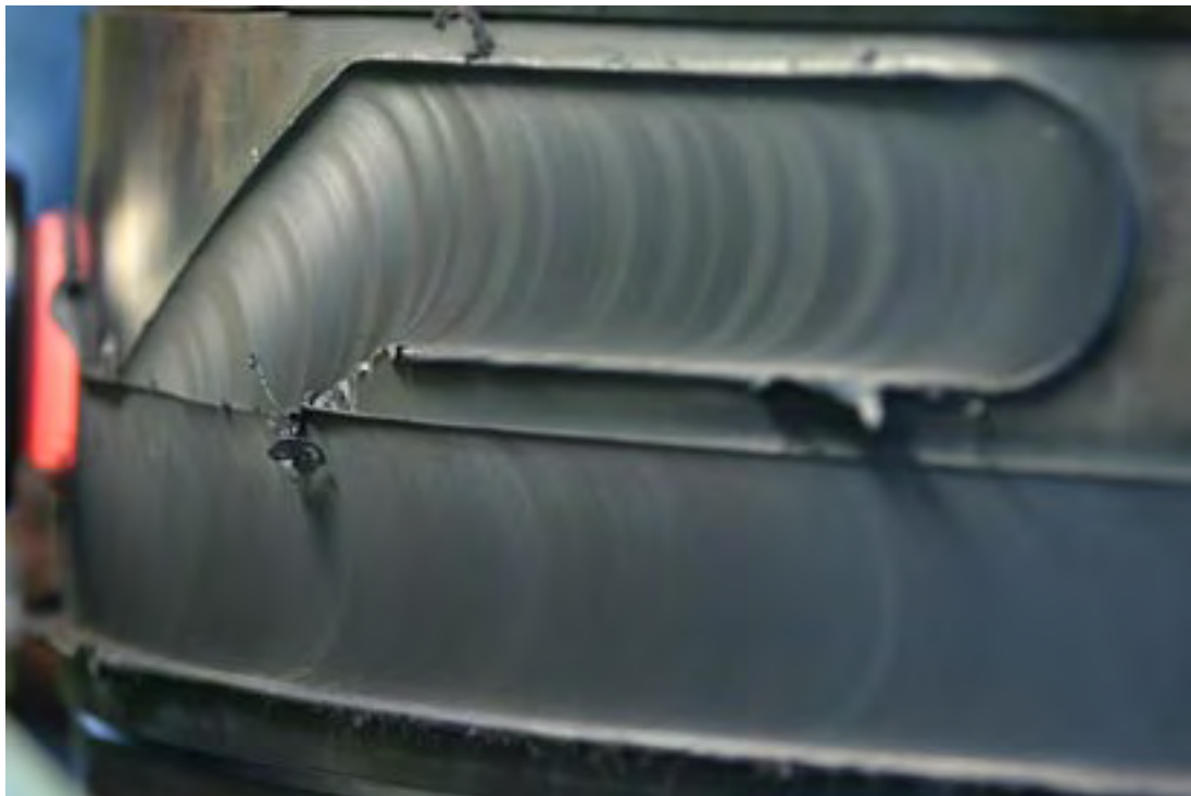
Figure 6-19. Start sequence and FSW tool on the way up to the parking position at the bottom weld.
