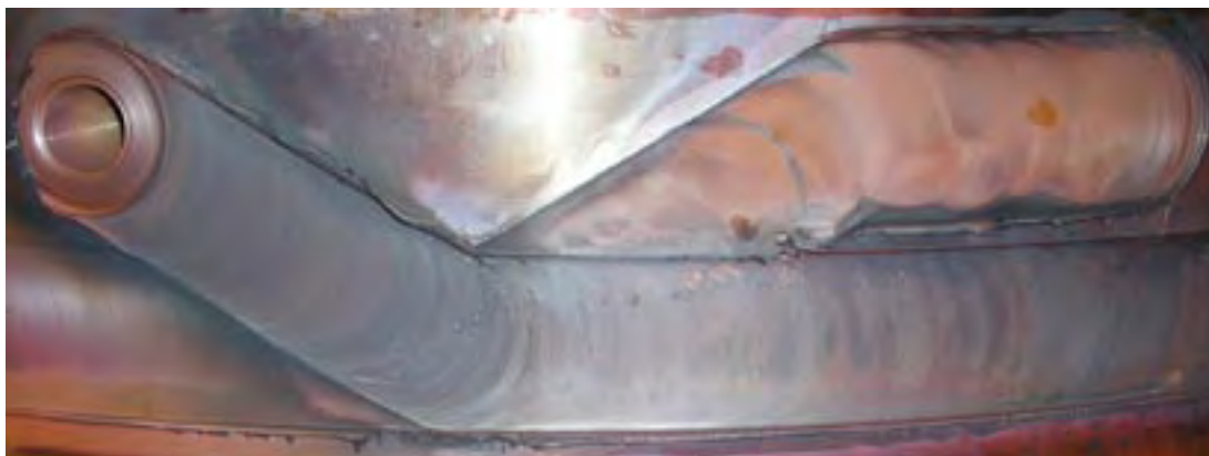
Figure 6-18. The start area (at right) and the exit hole (at left) above the joint line.
