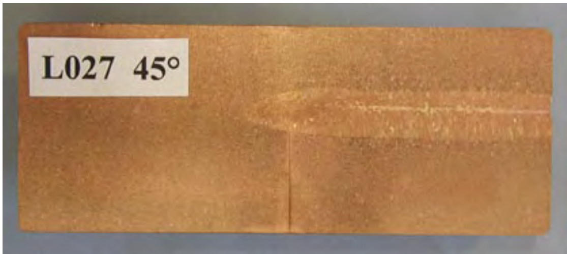
Figure 6-12. Lid weld L027. Cross-section of weld. The macrospecimen shows a weld depth of 66 millimetres and the weld has a root radius of 1.5 millimetres, which minimizes the risk of root defects.
