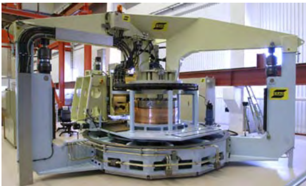
Figure 6-17. The FSW machine in the Canister Laboratory.
