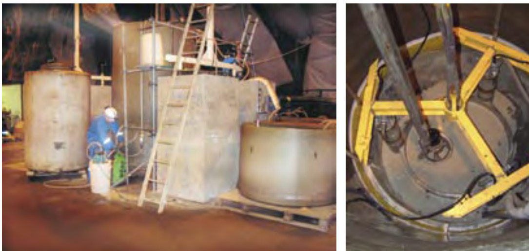
Figure 10-4. The photo at the left shows the experimental set-up used in the slurring test – slurring is done in the tank in the middle. The photo at the right shows how the bentonite is slurred by means of a salt solution.
