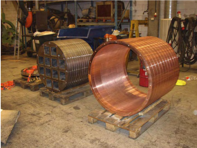
Figure 5-7. Part of cast insert and copper tube for compression testing.
