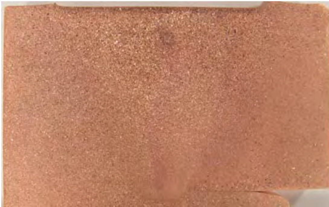
Figure 6-20. Macrosection of FSW weld showing the fine-grained microstructure that is obtained.
