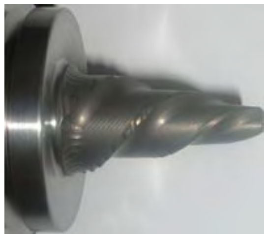
Figure 6-15. Schematic drawing of the FSW process. Figure 6-16. The FSW tool.
