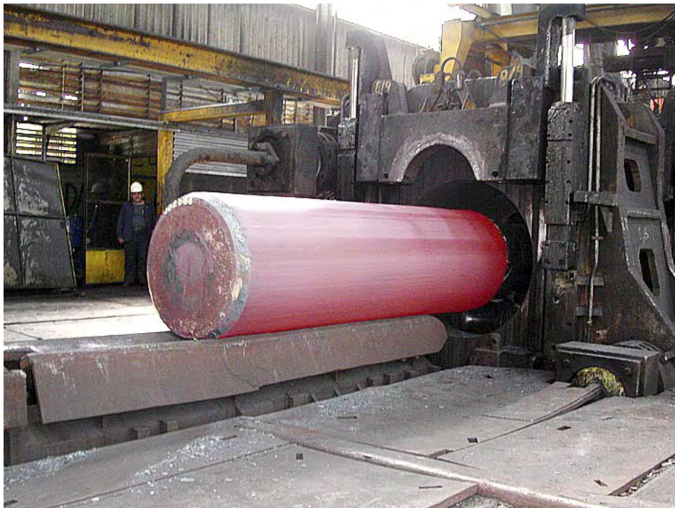
Figure 5-12. Fabrication of copper tube with integral bottom by pierce and draw processing.
