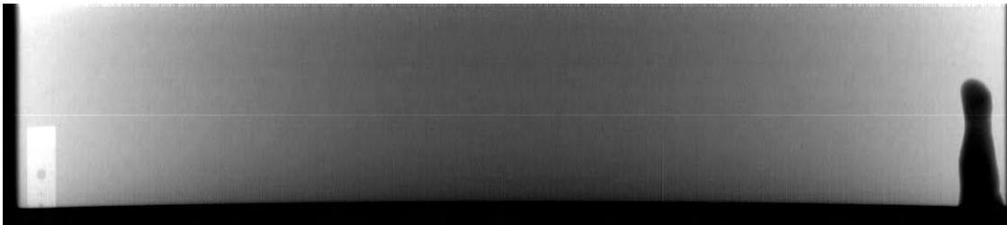
Figure 6-8. Radiograph of weld TB 122. If welding is interrupted, the cavity (key hole) in the material that constantly surrounds the beam during welding is retained. This provides an image of the shape of the beam. The round shape is important for avoiding root defects.
