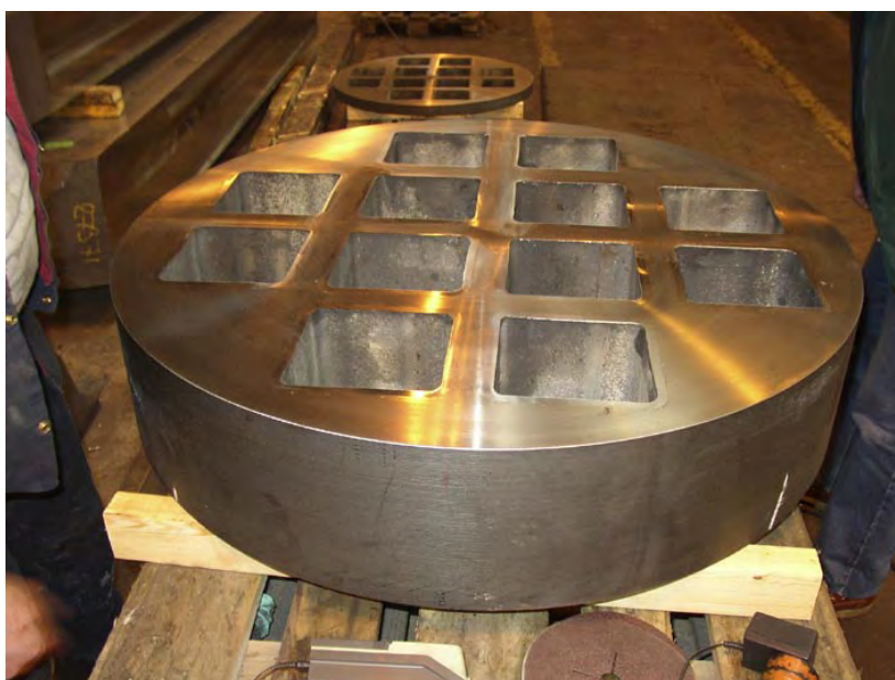
Figure 5-4. Discs cut from cast insert for material testing.
