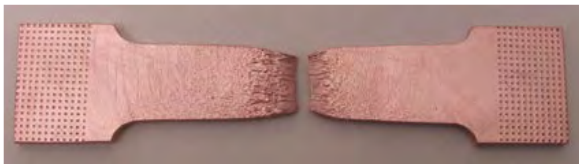
Figure 6-14. Tensile specimen from lid weld L028. Rotational position 310°.
