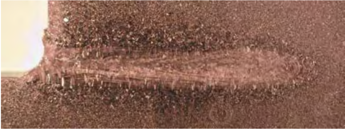
Figure 6-7. Macrospecimen from weld TB 122. Welding test with oscillating beam.
