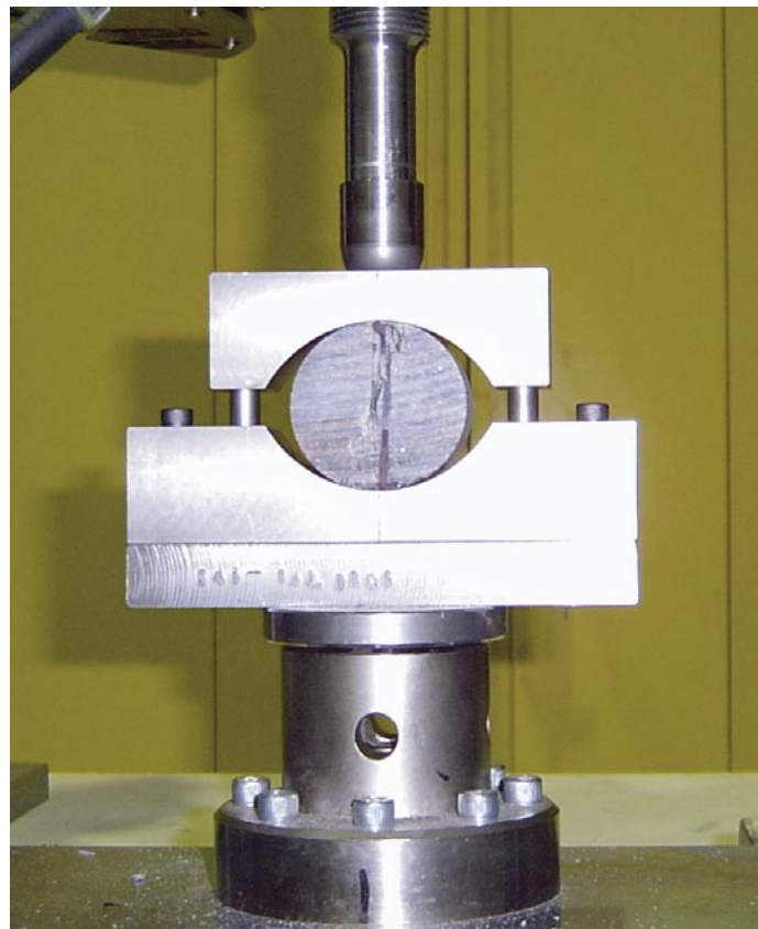
Figure 3-1. Curved bearing blocks for the indirect tensile test. The specimen in the picture does not belong to the test series in this report.
