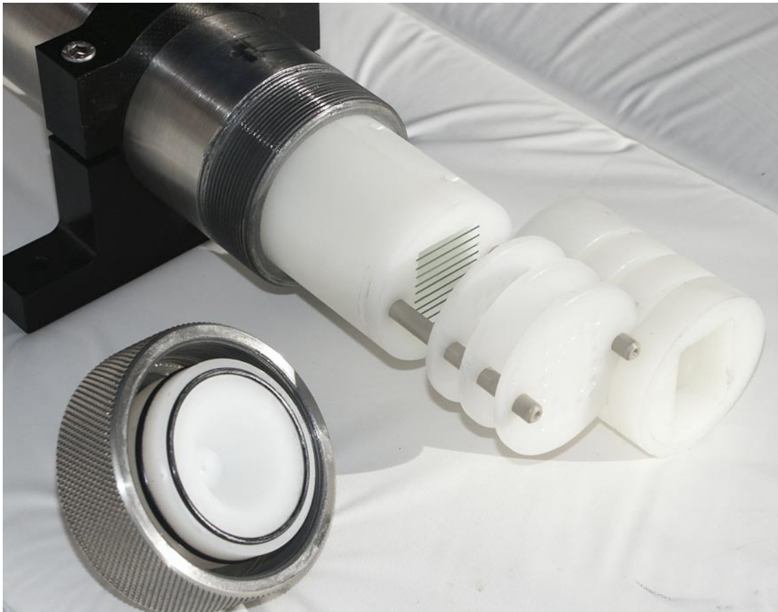
Figure 4-18. The flow cell that was used to grow biofilms. Glass slides were exposed to circulating groundwater from borehole KJ0052F03 for about 15 months.
