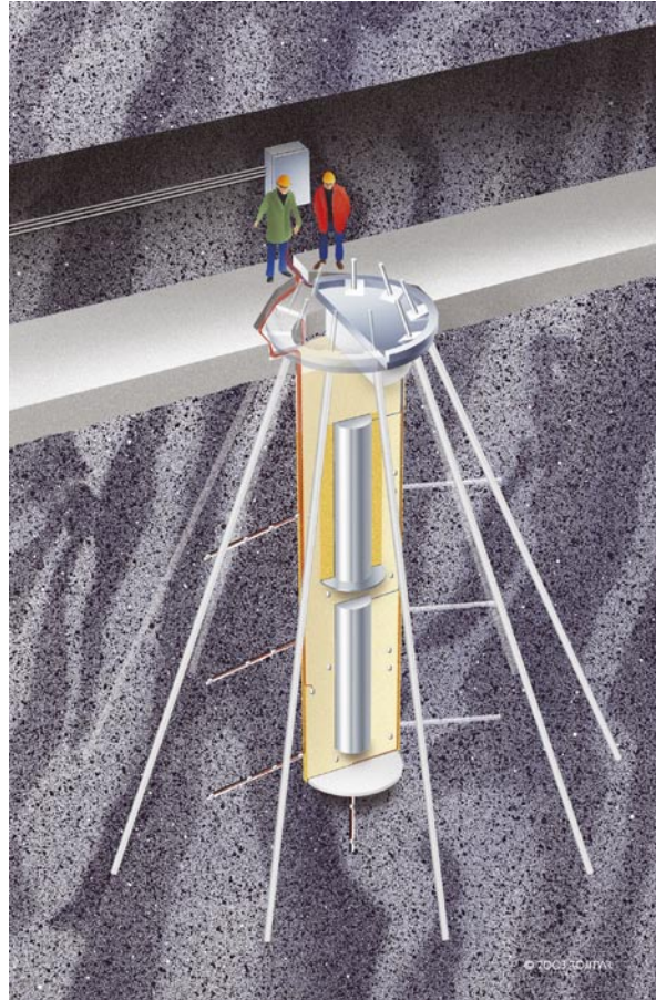
Figure 2-25. Principle design and experimental set-up of the Temperature Buffer Test.
