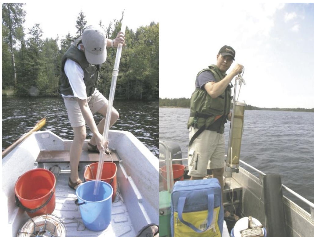
Figure 3-1. The “Rambergör” (left) was used to sample phytoplankton and the Limnos catcher (right) was used to sample zooplankton.
