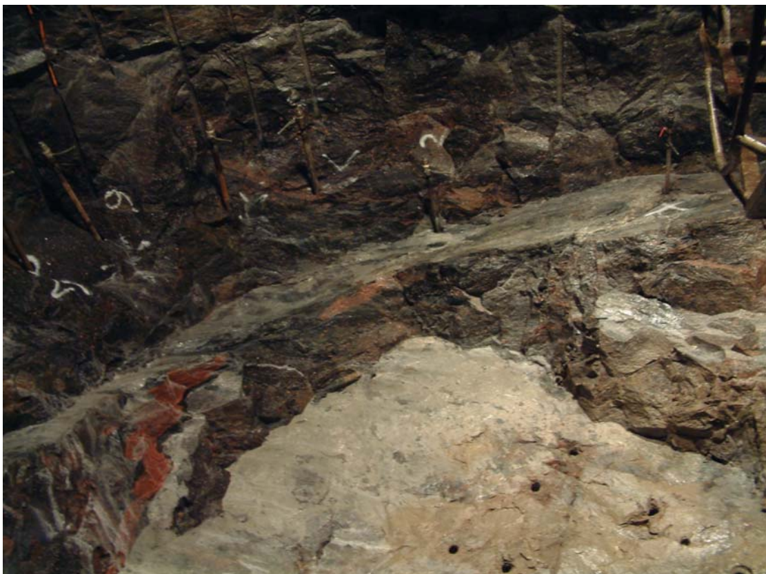
Figure 29. Larger scale exposures of diagonal (set 3a) sub-perpendicular (set 2) and perpendicular (set 1) joints at ch. 39-41m, and ch. 58-59m respectively.
