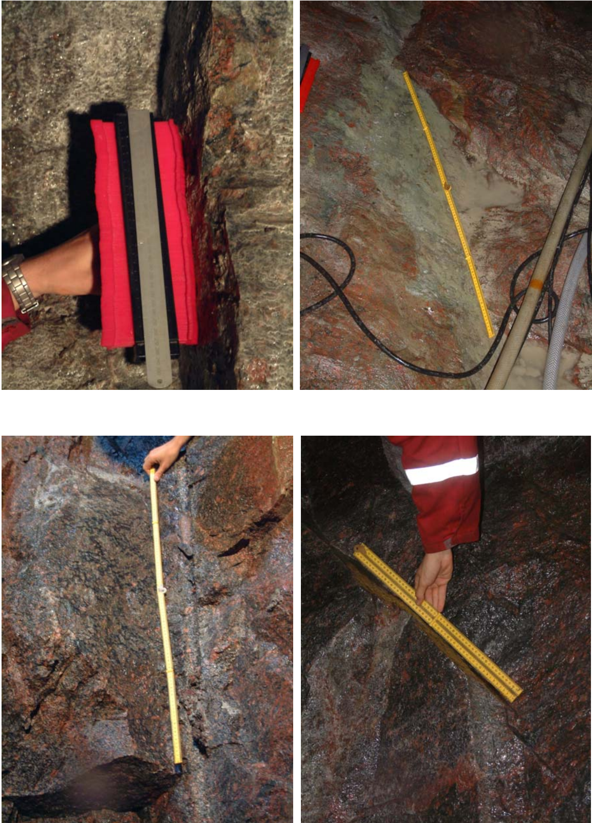
Figure 31. A selection of joint roughness illustrations: from top left, clockwise: set 2 (73m), set 3b (66m), set 3b (66m) and set 3b (62m).
