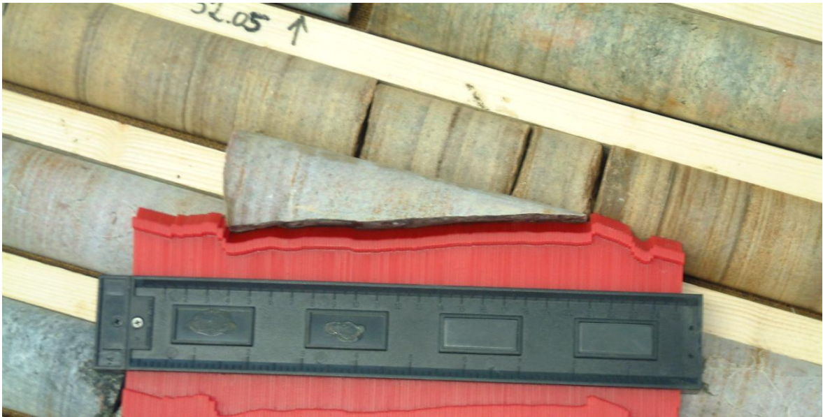
Figure 4-2. Example of a/L and JRC estimation, set 2 ( JRC \approx 4-6 ).
