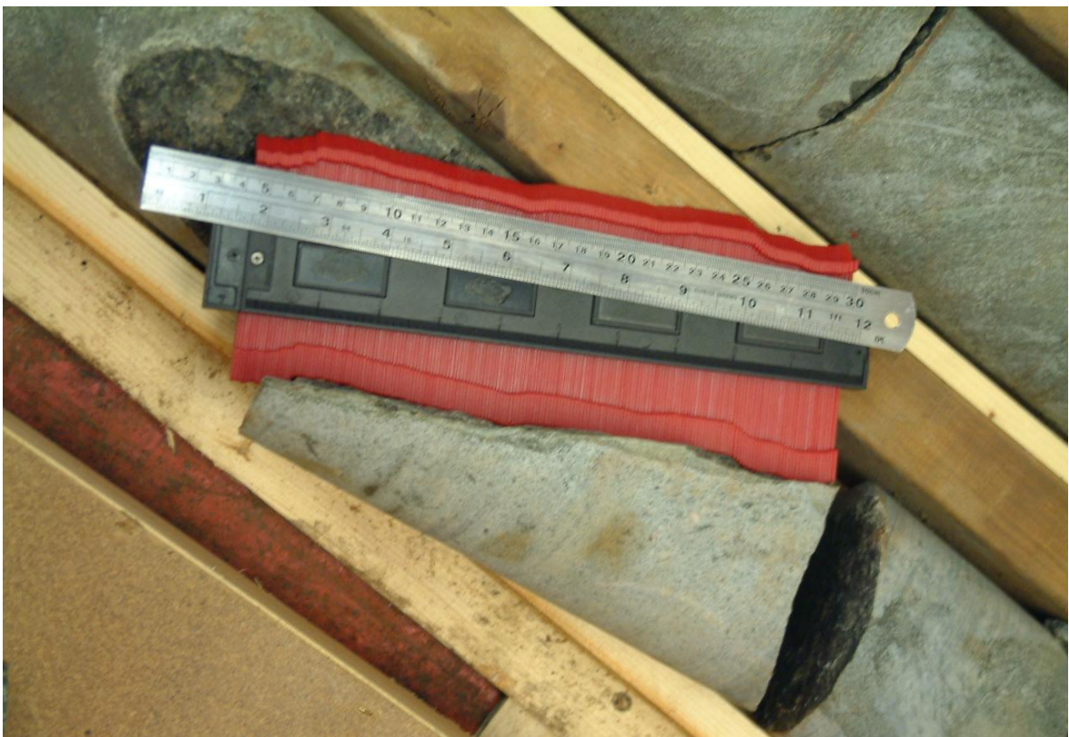
Figure 4-3. Example of a/L and JRC estimation, set 2 ( JRC \approx 6-8 ).
