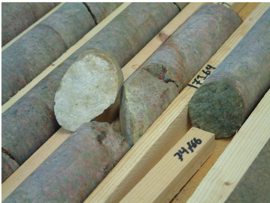
Figure 7. Typical appearance of KA3376B01 core, and details of three joint sets with J_a = 3 to 4.
