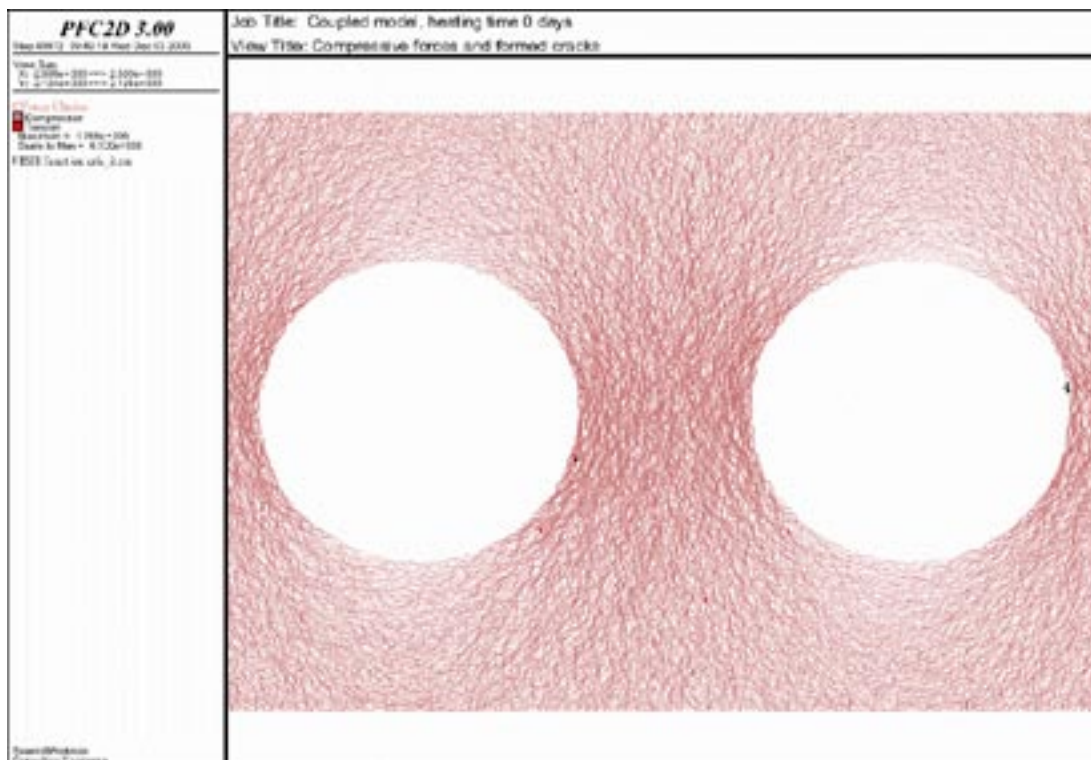
Figure 4-3. Forces between the particles. Vector width is proportional to the magnitude of the effective force. Pillar area is loaded mainly in compression. Upper part of the hole wall is nearly unloaded or in tension (black=tension, red=shear).
