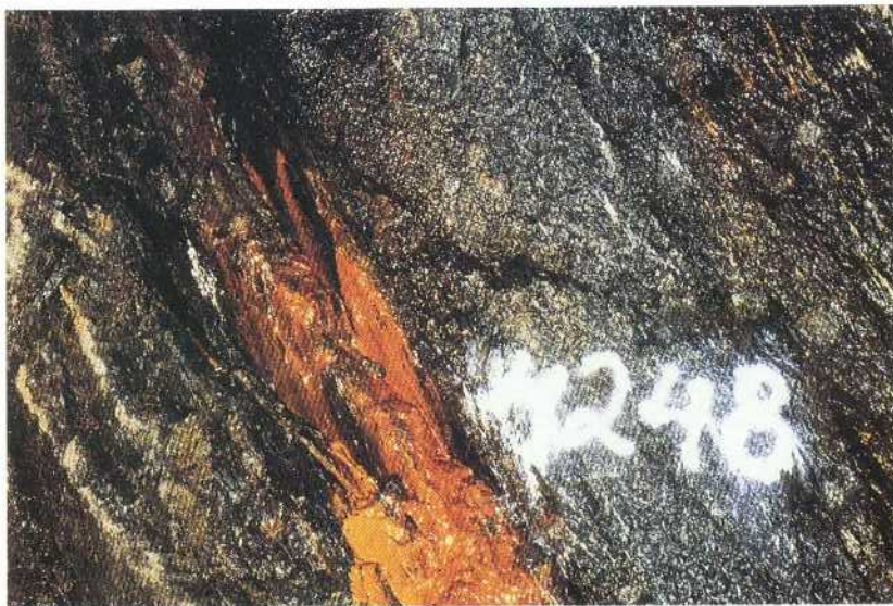
Point leakage (∇) from a contact leptite/amphibolite in a crush zone. 4/248
