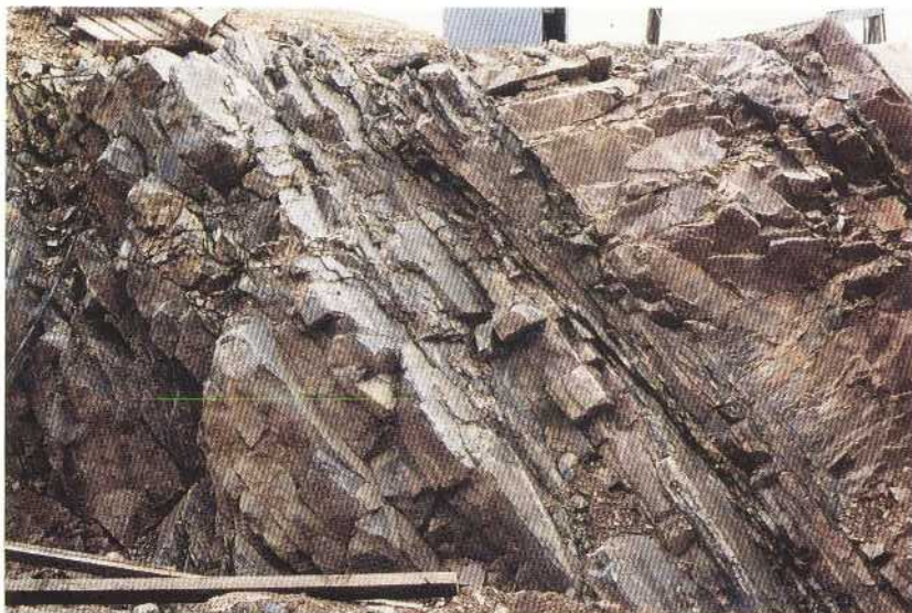
Open cut Granån. Thin slaty fracture zone=K2 in leptite,
